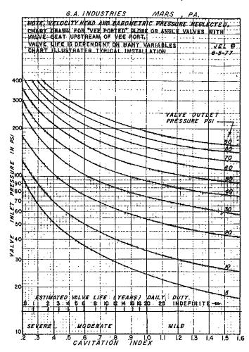
Cavitation damage is only one of four principle types of damage which can occur to a valve. A valve can also sustain abrasive particle damage, impingement erosion, and sometimes a combination of these conditions. Many times impingement erosion is interpreted as cavitation damage. These problems will not be elaborated on at this time.
