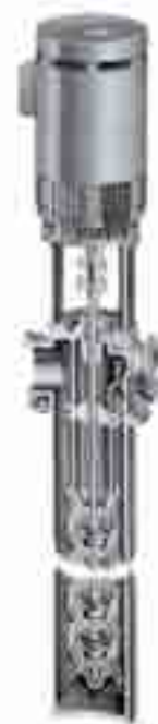
Figure 11. Typical Vertical Can-Type Pump.
