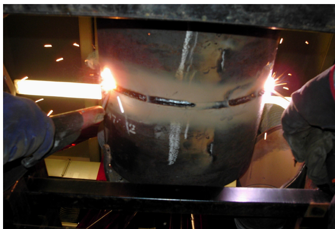
Figure 5 – SMAW welding on P23
