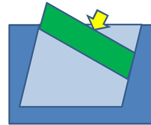
**If Rule #1 is in charge, regardless whether the parts are rectangles or parallelograms (so regardless of perpendicularity error) assembly is always possible as long as MMC dimensions for puck and pocket do not conflict with each other**
