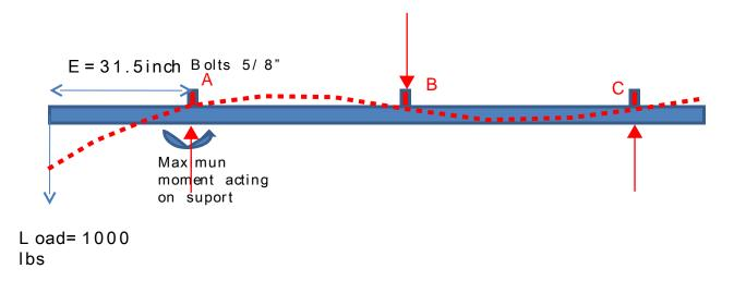
How i must to calculate the stress on bolt, stress due to bending S = Moment/ Wx(bolt) or S = Axial load/ area bolt
