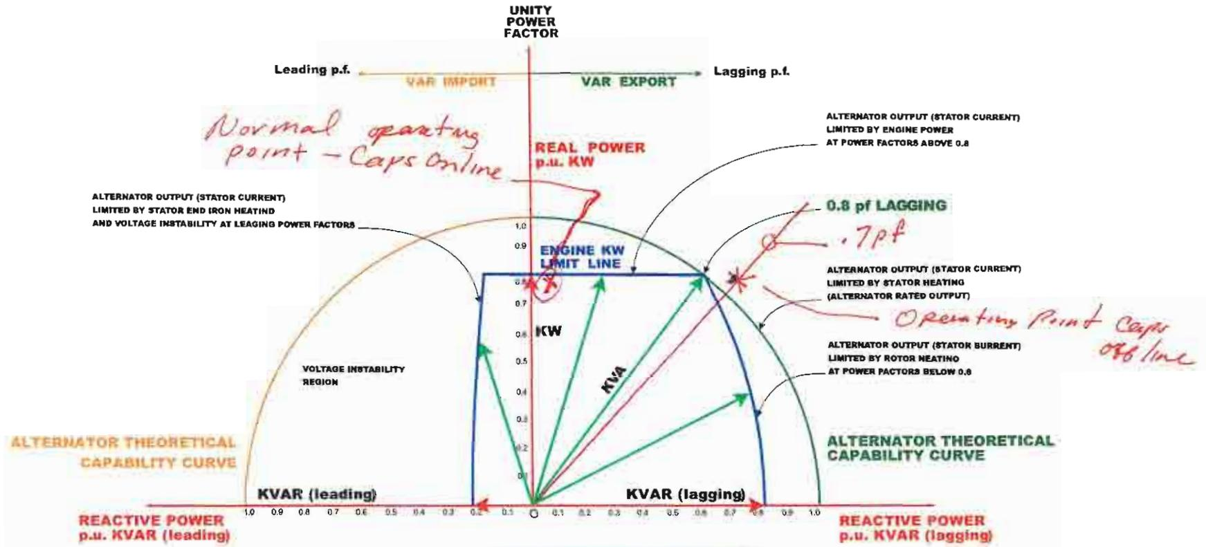
LEADING POWER FACTOR RESULTS IN THE ALTERNATOR BEING UNDER-EXCITED - LOW ROTOR (FIELD) CURRENT
