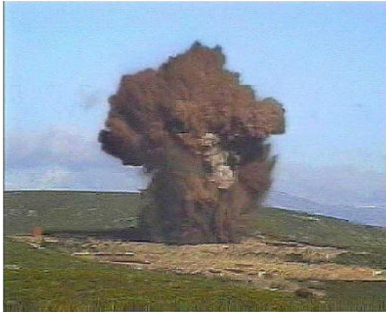
Figure 11: Full scale burst tests on X100 line pipe
