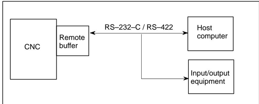
When the remote buffer is connected online to the host computer, fast and reliable DNC operation is possible.
