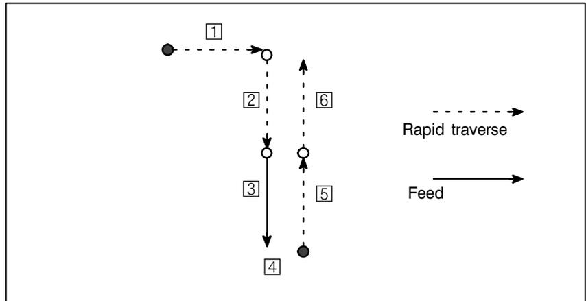
Fig. 5.5 (b) Single block during canned cycle
