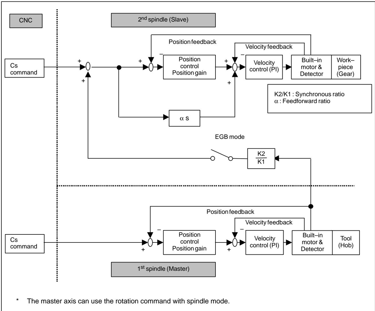
Fig. 20.8.3 (a) Block diagram for Spindle EGB control
