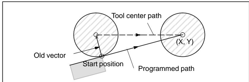
This command changes the mode of the equipment from the cutter compensation mode to the cancel mode.
