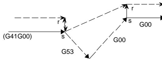
Example 2: When CCN (bit 2 of parameter No. 5003) = 1 and all-axis machine lock is applied [FS15 type]
