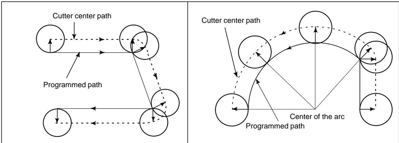
Fig. 14.11 (b) Normal direction control left (G41.1)
