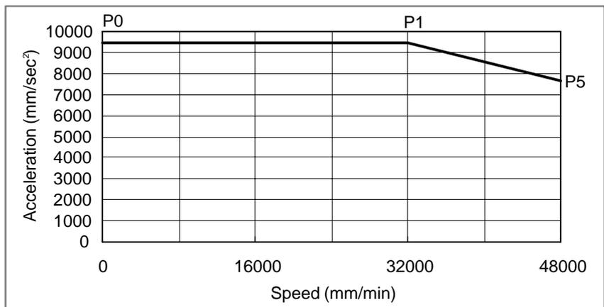
Fig.19.10(l) Acceleration pattern in case of – move and acceleration
