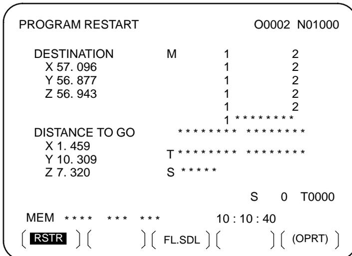
DESTINATION shows the position at which machining is to restart. DISTANCE TO GO shows the distance from the current tool position to the position where machining is to restart. A number to the left of each axis name indicates the order of axes (determined by parameter setting) along which the tool moves to the restart position.
