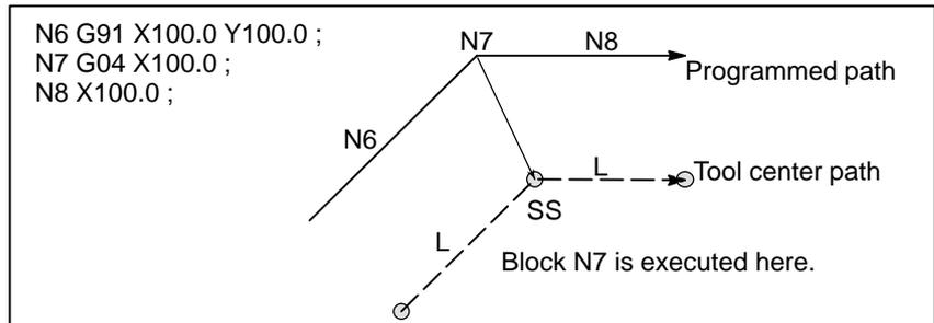
However, when the move distance is zero, even if the block is commanded singly, tool motion becomes the same as that when more than one block of without tool movement are commanded, which will be described subsequently.
