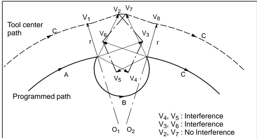
(2) If the interference occurs after correction (1), the tool is stopped with an alarm.
