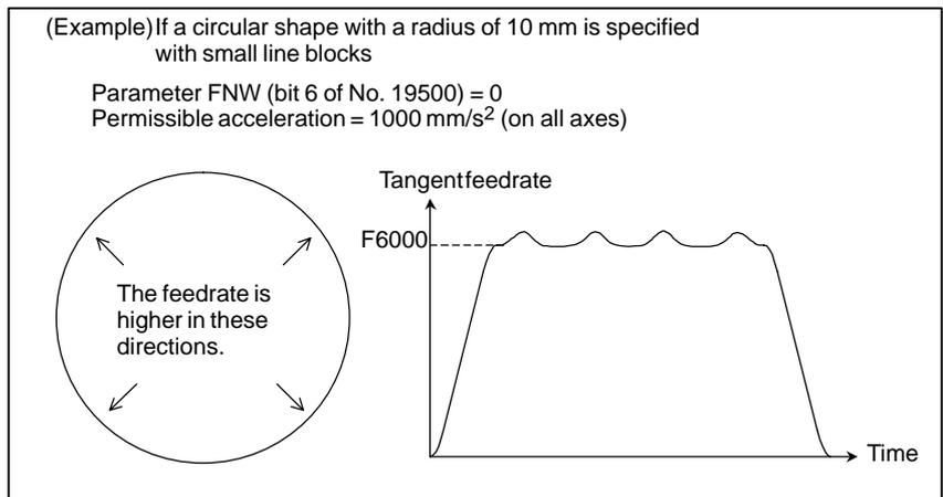
If "1" is set, the feedrate is determined with not only the condition that the permissible acceleration on each axis is not exceeded but also the condition that the deceleration feedrate is constant regardless of the travel direction if the shape is the same.
