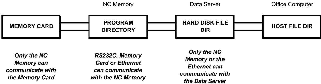
To use the DATA SERVER the I/O Channel on the SETTING page must be set to 5. If the machine does not have a data server this setting must be "9" to communicate with the embedded ethernet
