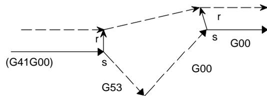
Example 3: When CCN (bit 2 of parameter No. 5003) = 1 and specified-axis machine lock is applied [FS15 type]
