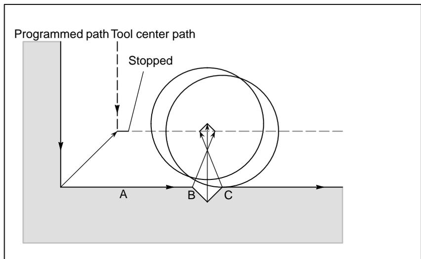
Like (1), P/S alarm is displayed because of the interference as the direction is reverse in block B.
