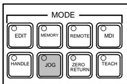
The tool length offset value can be measured by manually moving the tool until it touches the workpiece or a reference block. For details of this operation, refer to the manual supplied by the machine tool builder.
