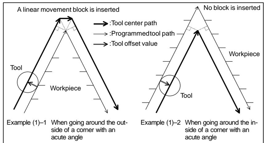
**Fig. 22.5.1 (e) Operation in the compensation mode (1)-1, 2**
