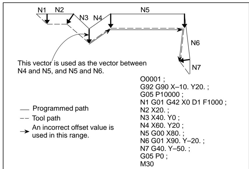
(2) When G00 is specified with bit 7 of parameter SG0 No. 8403 set to 1, the following points should be noted:
