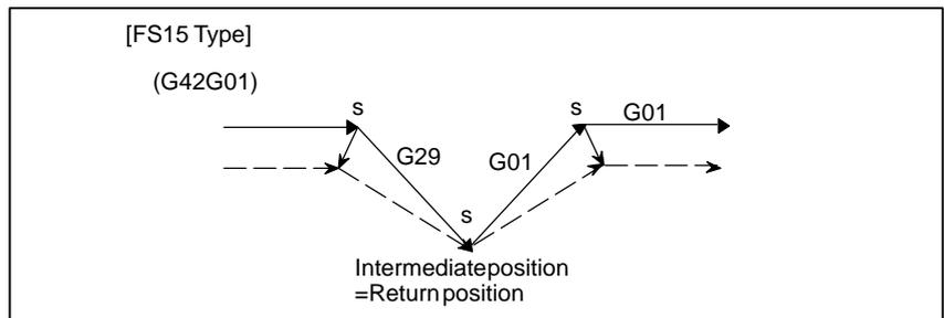
(4) G29 specified in offset mode (with movement to an intermediate position and reference position not performed)
