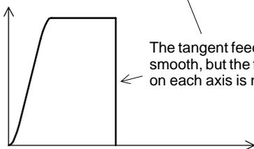
The tangent feedrate is smooth, but the feedrate on each axis is not.
