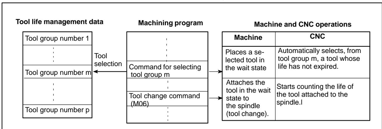
Fig. 10.2 (b) Tool Selection by Machining Program
