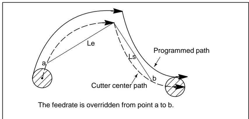
**Fig. 5.4.2.1 (c) Override Range (Arc to Arc)**
