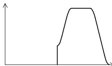
The method of deceleration based on the feedrate difference differs depending on the setting made for parameter FNW (bit 6 of No. 19500). If "0" is set, the largest feedrate that does not exceed the permissible feedrate difference set for parameter No. 8410 is assumed to be the deceleration feedrate. In this case, the deceleration feedrate differs if the travel direction differs, even if the shape is the same.
