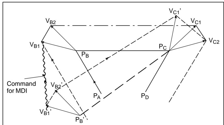
When position  $P_A$ ,  $P_B$ , and  $P_C$  are programmed in an absolute command, tool is stopped by the single block function after executing the block from  $P_A$  to  $P_B$  and the tool is moved by MDI operation. Vectors  $V_{B1}$  and  $V_{B2}$  are translated to  $V_{B1}'$  and  $V_{B2}'$  and offset vectors are recalculated for the vectors  $V_{C1}$  and  $V_{C2}$  between block  $P_B$ - $P_C$  and  $P_C$ - $P_D$ .
