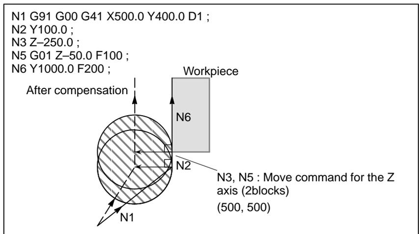
As the block with sequence No. N2 has the move command in the same direction as that of the block with sequence No. N6, the correct compensation is performed.
