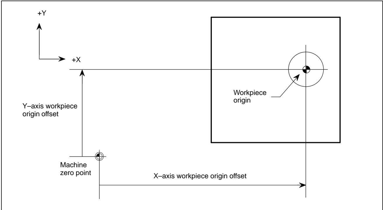
In the above case, the workpiece origin is located at the center of a hole in the workpiece. A measurement probe having a sensor at its tip is used to measure the positions of three arbitrary points on the circumference of the hole. The three points prescribe a unique circle, the center of which is set as the X-/Y-axis workpiece origin. Set bit 4 (WMH) of parameter No. 5007 to 1 before starting the measurement.
