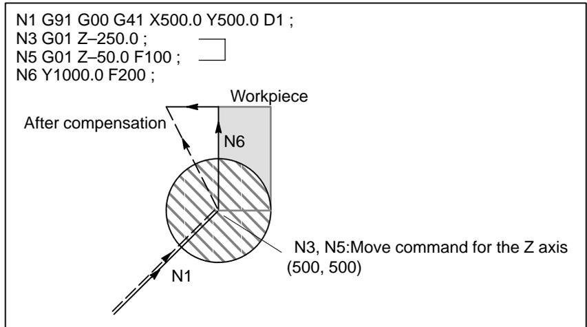
The move command in the same direction as that of the move command after the motion in Z axis should be programmed.
