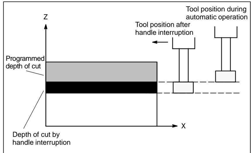
**Fig. 1.3 (c) Handle Interruption for Automatic Operation**
