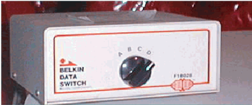
The front view of a Belkin Data Switch box showing the switch dial for the four machines supported
