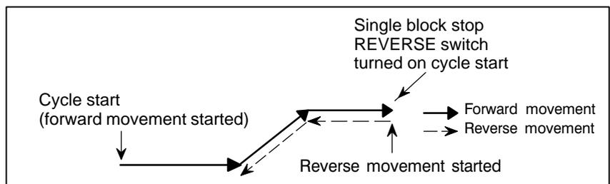
In the case of 3) above, the tool starts reverse movement at the position of a feed hold stop when the cycle start switch is pressed.
