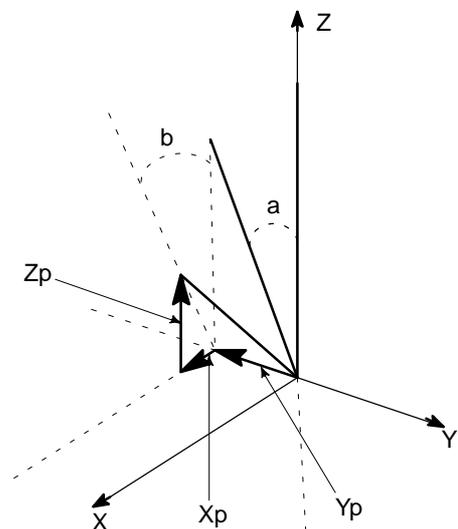
In the figures above, a, b, and c represent the positions (angles) of the A-axis, B-axis, and C-axis from the machine zero point; those values present when the tool axis direction handle feed mode is set or a reset occurs are used. To change the feed direction, reenter the tool axis direction handle feed mode, or press the reset key.
