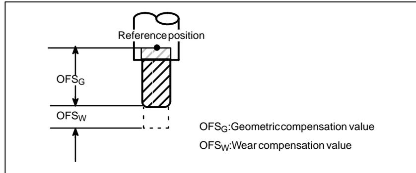
**Fig. 14.8 (a) Geometric compensation and wear compensation**
