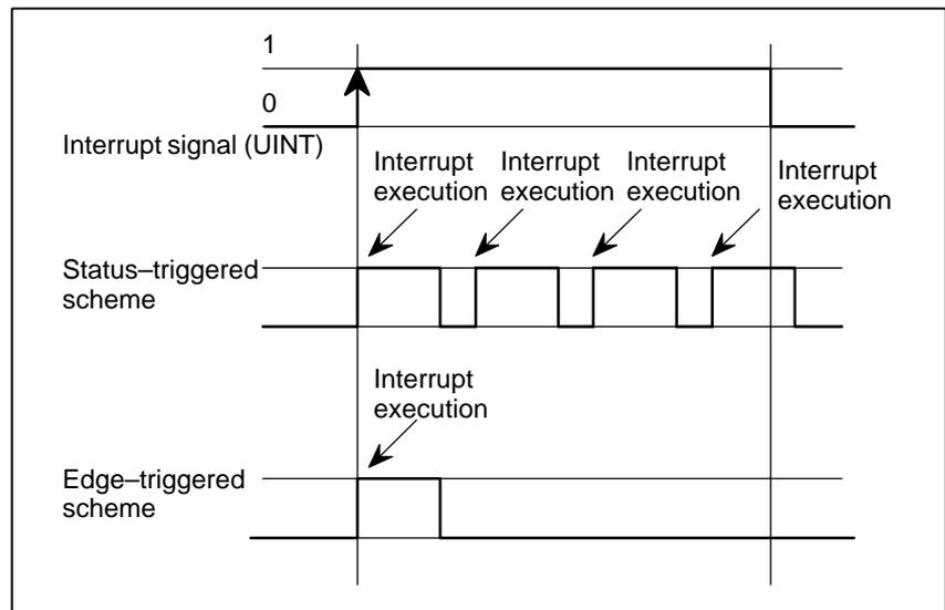
In the above example, an interrupt is executed four times when the status-triggered scheme is used; when the edge-triggered scheme is used, the interrupt is executed just once.
