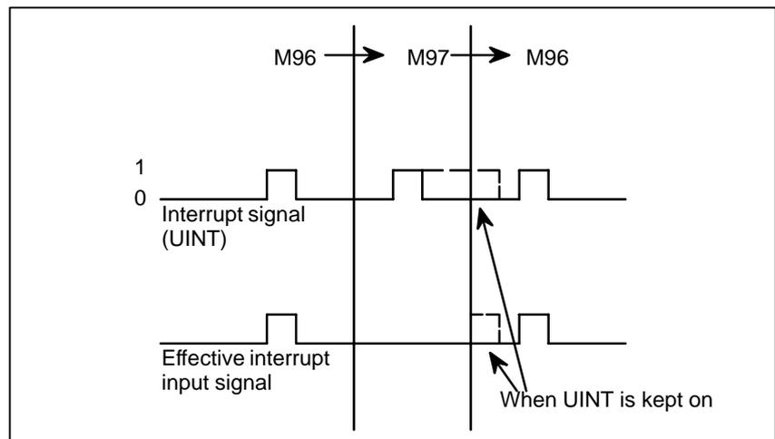
The interrupt signal (UINT) becomes valid after M96 is specified. Even when the signal is input in M97 mode, it is ignored. When the signal input in M97 mode is kept on until M96 is specified, a custom macro interrupt is initiated as soon as M96 is specified (only when the status-triggered scheme is employed); when the edge-triggered scheme is employed, the custom macro interrupt is not initiated even when M96 is specified.
