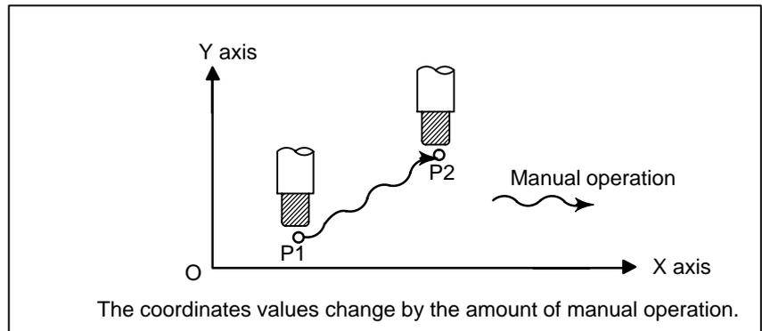
**Fig. 3.5 (a) Coordinates with the switch ON**
