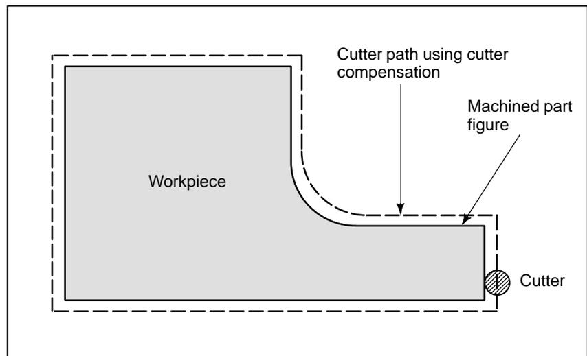
If radius of cutters are stored in the CNC (Data Display and Setting : see III-11), the tool can be moved by cutter radius apart from the machining part figure. This function is called cutter compensation.
