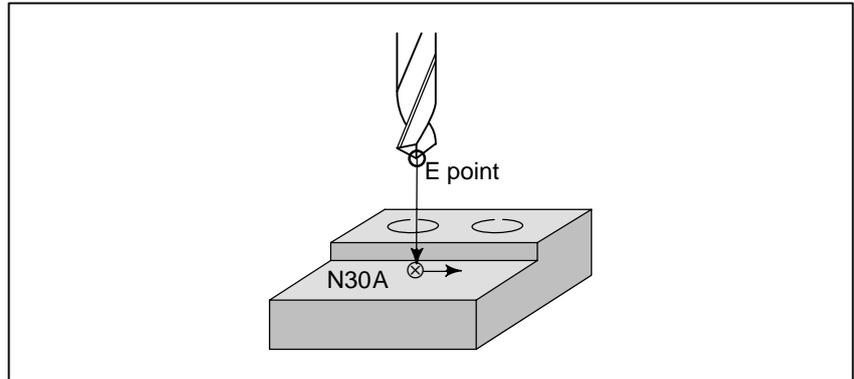
Upon completion of repositioning, the tool withdraw mode is cancelled, and the TOOL BEING WITHDRAWN LED goes off and restart N30.
