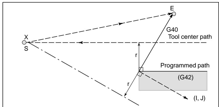
When an intersection is not obtainable, the tool comes to the normal position to the previous block at the end of the previous block.
