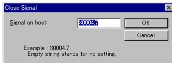
3. Enter the target PMC signal in the Signal on host text box, using the following format, then choose the  button.
