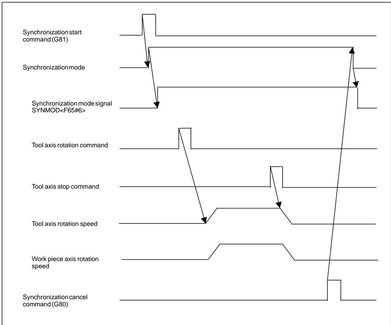
Fig. 20.8.3 (b) Example timing for starting/canceling synchronization
