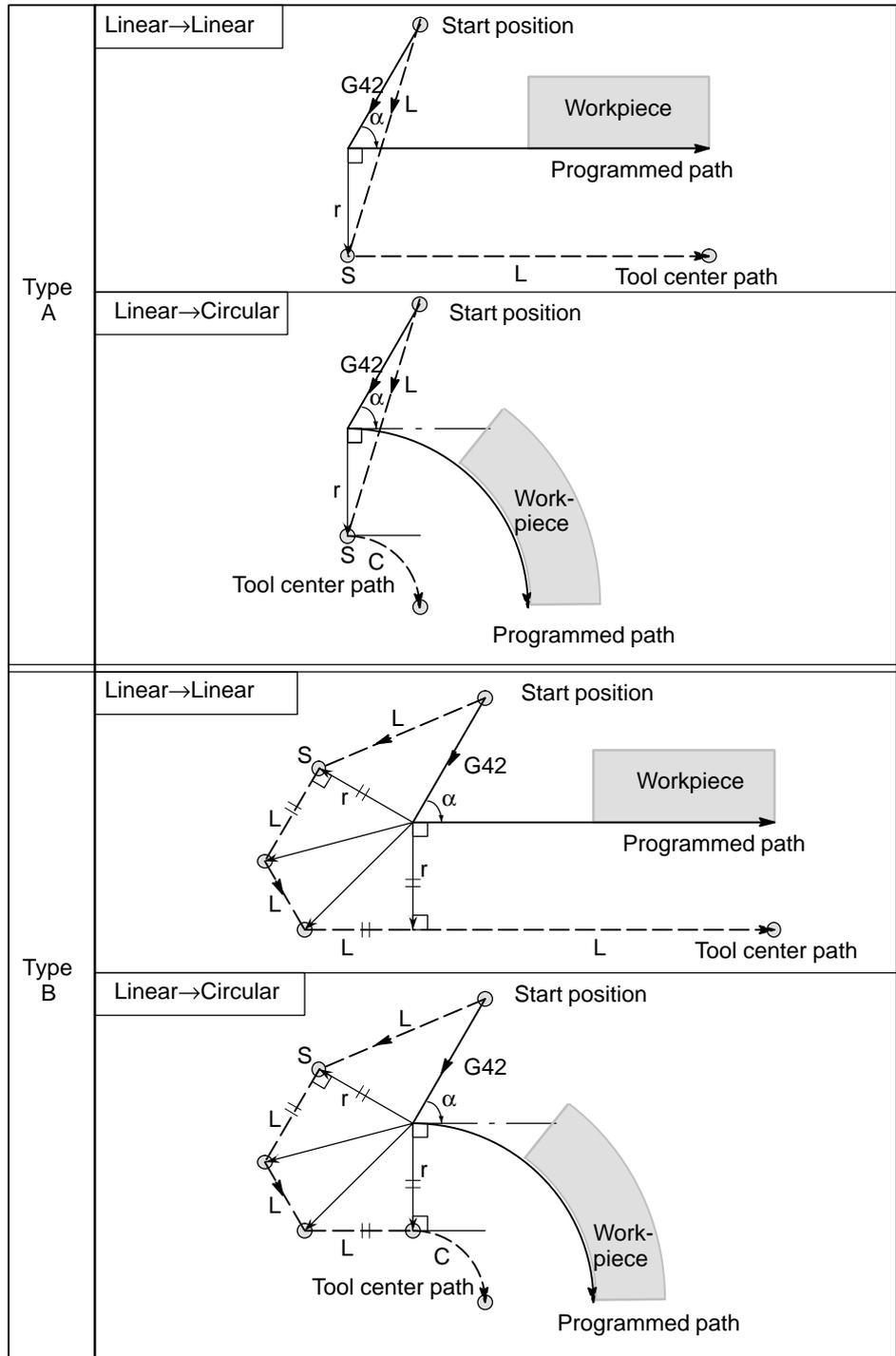
● **Tool movement around the outside linear→linear at an acute angle less than 1 degree ( $\alpha < 1^\circ$ )**
