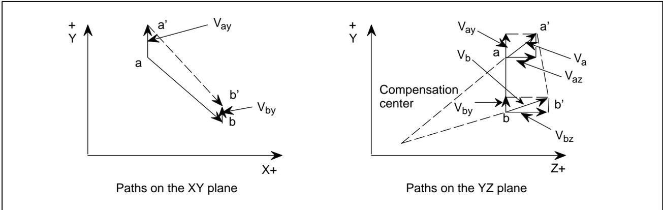
(Example 2) When the compensation axes are the Y- and Z-axes and circular interpolation is performed for the X- and Y-axes
