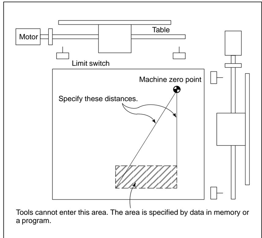
Besides strokes defined with limit switches, the operator can define an area which the tool cannot enter using a program or data in memory. This function is called stroke check (see III-6.3).
