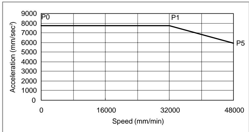
Fig.19.10(n) Acceleration pattern in case of – move and deceleration
