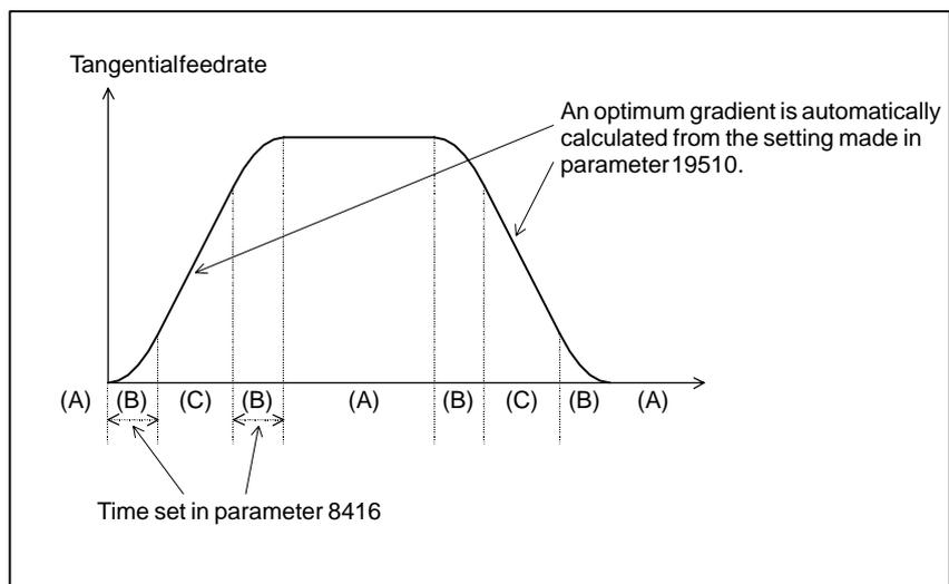
● **Method of determining the tangent acceleration**
