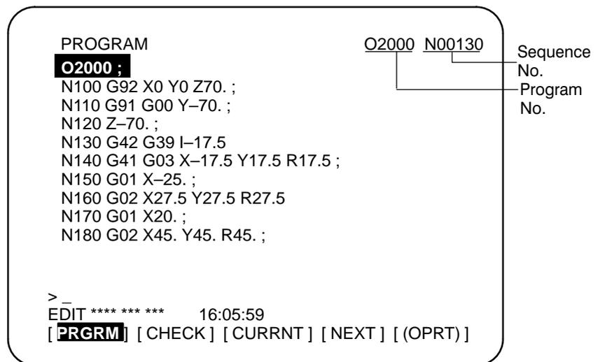
**The program number and sequence number displayed depend on the screen and are given below:**
