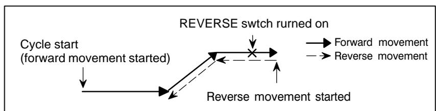
In the case of 2) above, the tool starts reverse movement at the position of a single block stop when the cycle start switch is pressed.
