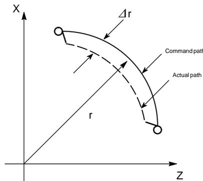
$$\Delta r = \frac{1}{2}(T_1^2 + T_2^2(1 - a^2))\frac{V^2}{r} \dots\dots (1)$$
