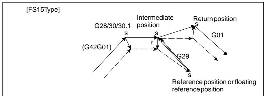
(b) For specification made other than immediately after automatic reference position return
