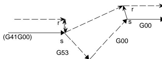
2 When G53 is specified for a compensation axis in cutter compensation mode, the vectors along the other axes are also canceled. (This also applies when CCN (bit 2 of parameter No.5003) is set to 1. When the FS15 type is used, only the vector along a specified axis is canceled. Note that the FS15 type cancellation differs from the actual FS15 specification in this point.)
