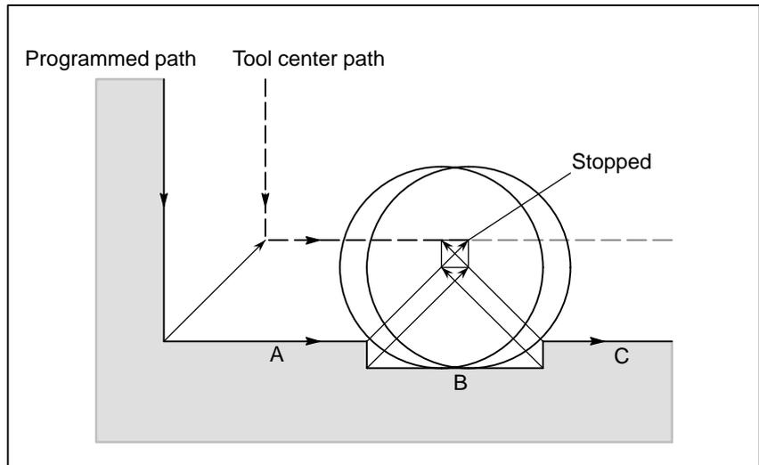
There is no actual interference, but since the direction programmed in block B is opposite to that of the path after cutter compensation the tool stops and an alarm is displayed.
