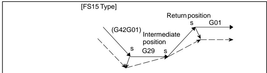
(2) G29 specified in offset mode (with movement to an intermediate position not performed)
