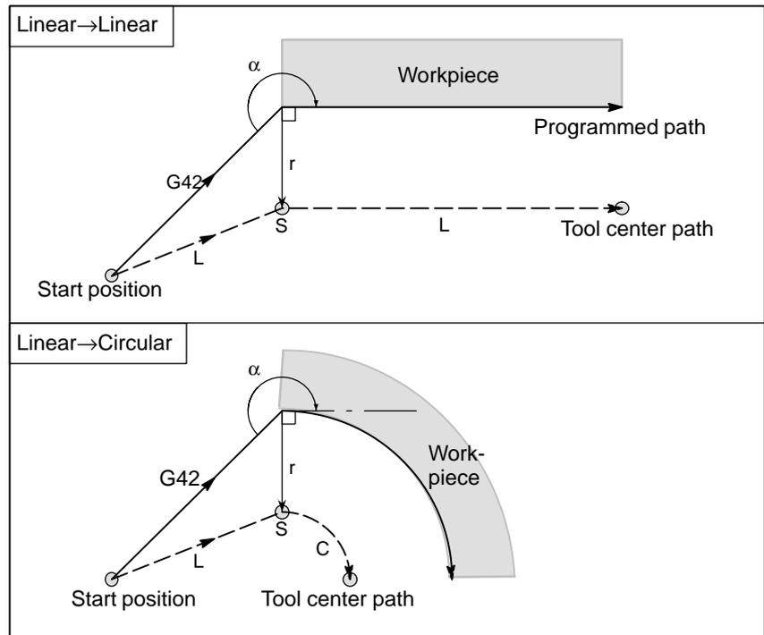
● **Tool movement around the outside of a corner at an obtuse angle ( $90^\circ \leq \alpha < 180^\circ$ )**
