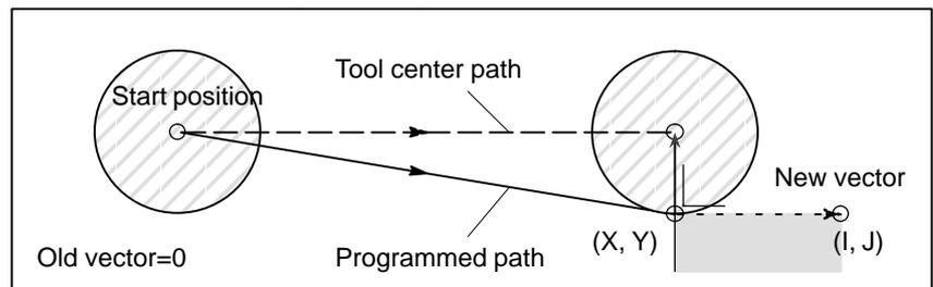
Unless otherwise specified, (I, J) are assumed to be equal to (X, Y). When the following command is specified, a vector perpendicular to a line connecting the start position and position (X, Y) is created.
