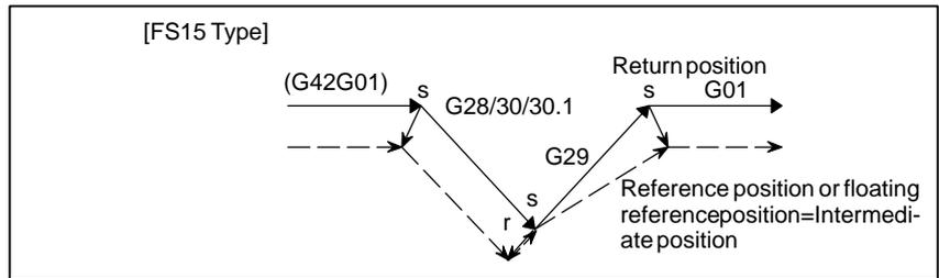
(b) For specification made other than immediately after automatic reference position return
