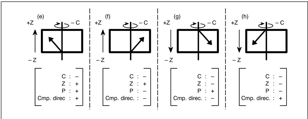
Fig. 20.8.3 (c) Direction of helical gear compensation
