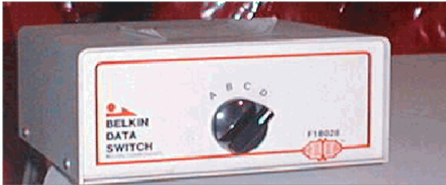
The front view of a Belkin Data Switch box showing the switch dial for the four machines supported
