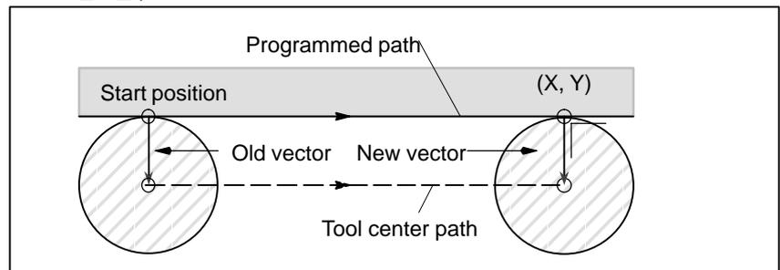
In the case of G00, however, each axis moves independently at the rapid traverse rate.
