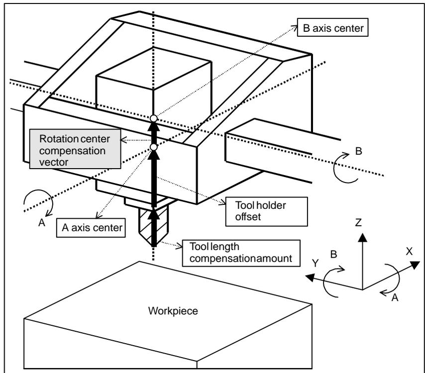
**Fig. 22.4 (c) Compensation of Rotation Centers of Two Rotation Axes**
