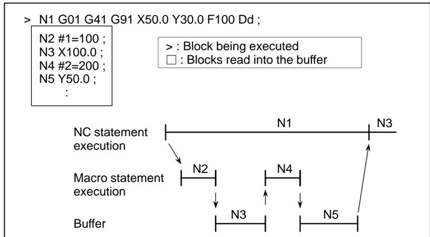
When N1 is being executed, the NC statements in the next two blocks (up to N5) are read into the buffer. The macro statements (N2, N4) between N1 and N5 are processed during execution of N1.
