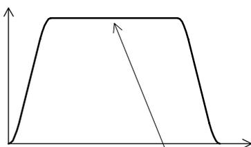
The deceleration based on the feedrate difference is used.
