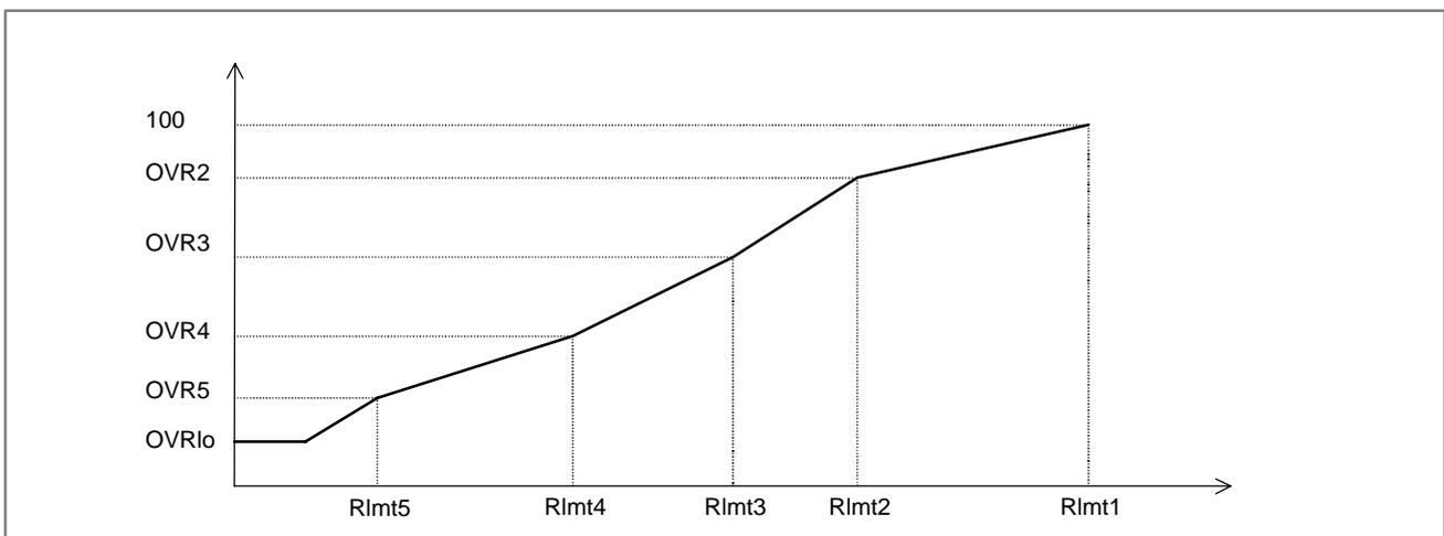
If the calculated override is lower than the lower limit set in the corresponding parameter, it is clamped to the lower override limit.
