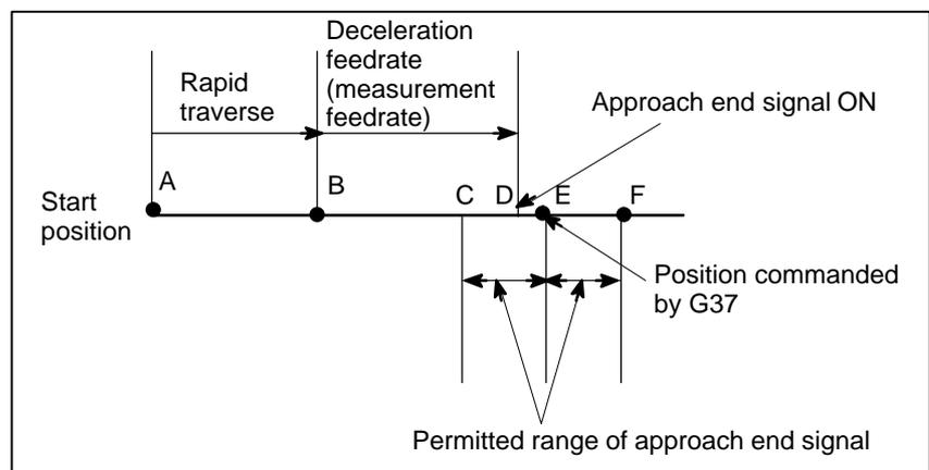
**Fig. 14.2 (b) Tool movement to the measurement position**
