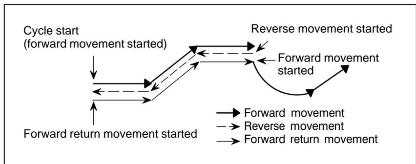
If the tool moves in the reverse direction after a feed hold stop, the tool stops forward return movement at the position of the feed hold stop, then resumes forward movement. If the tool moves in the reverse direction after a single block stop, the tool also stops forward return movement at the position of the single block stop.
