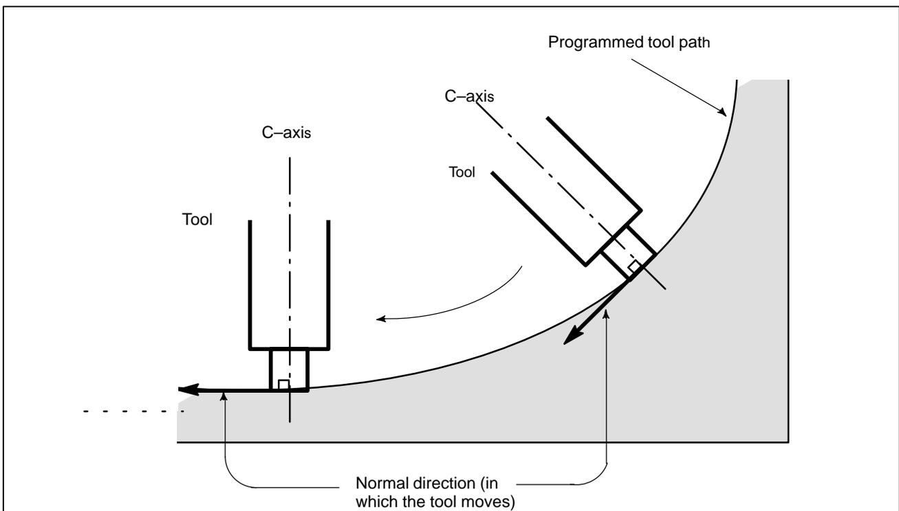
Fig. 14.11 (a) Sample Movement of the tool
