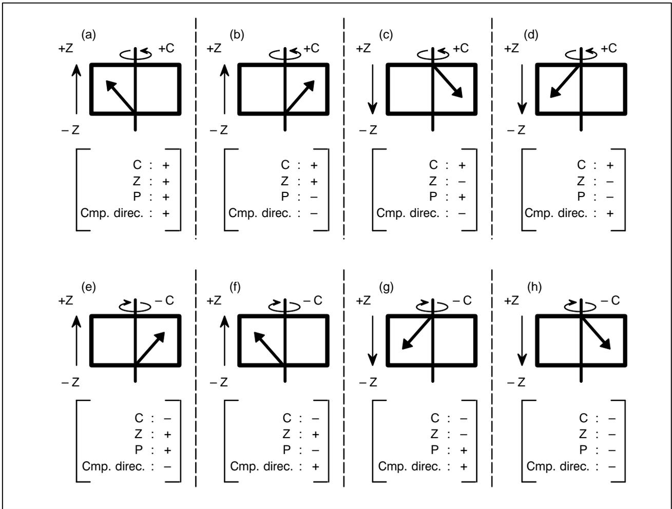
(2) When bit 2 (HDR) of parameter No.7700 is 0. (Items (a) to (d) are the same as for (1))
