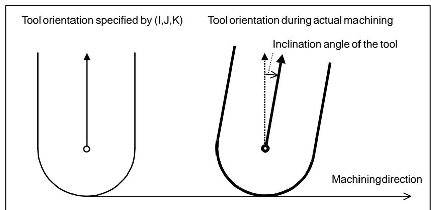
Example: For machining with the tool tilted toward the machining direction by 2 degrees, specify the following:
