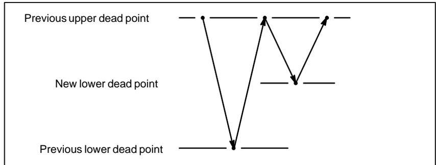
The tool first moves to the previous lower dead point, then to the upper dead point, and finally to the new lower dead point.
