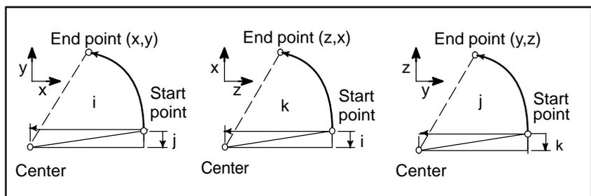
I0,J0, and K0 can be omitted. When  $X_p$ ,  $Y_p$ , and  $Z_p$  are omitted (the end point is the same as the start point) and the center is specified with I, J, and K, a 360° arc (circle) is specified.
