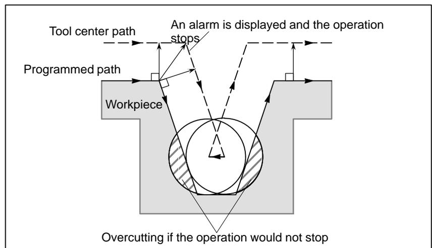
● **Machining a step smaller than the tool radius**
