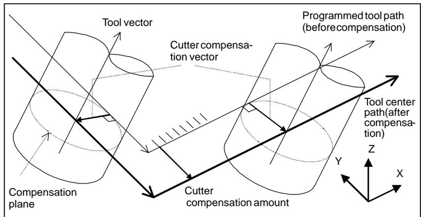
Fig. 22.5.1 (a) Tool side compensation
