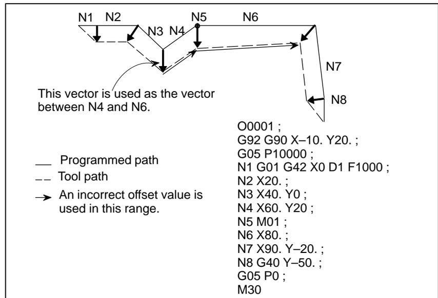
(Example 2) When the following program is executed for machining with offset value D1 set to 10 mm, the start point of N5 is determined by the vector created between N3 and N4. If the simplified G00 execution function is enabled (by setting bit 7 of parameter SG0 No. 8403 to 1), a correct vector can be obtained at the intersection of N4 and N5.
