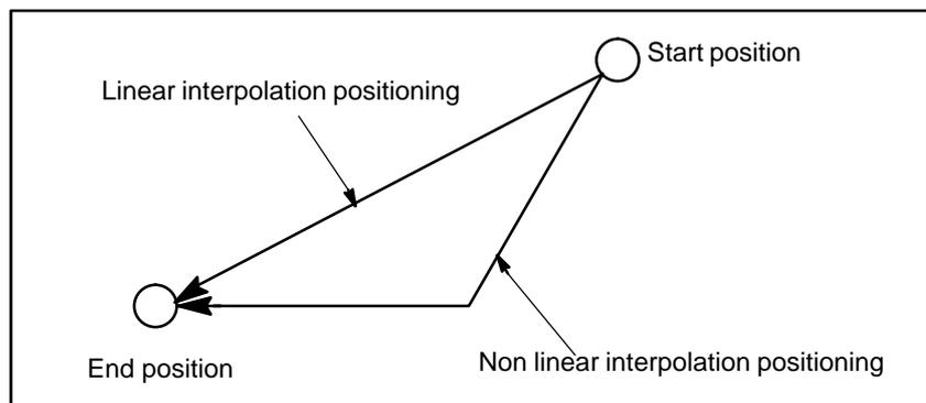
The rapid traverse rate in G00 command is set to the parameter No. 1420 for each axis independently by the machine tool builder. In the positioning mode actuated by G00, the tool is accelerated to a predetermined speed at the start of a block and is decelerated at the end of a block. Execution proceeds to the next block after confirming the in-position.
