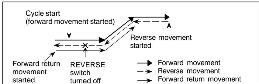
In the case of 2) above, the tool starts forward return movement at the position of a single block stop when the cycle start switch is pressed.
