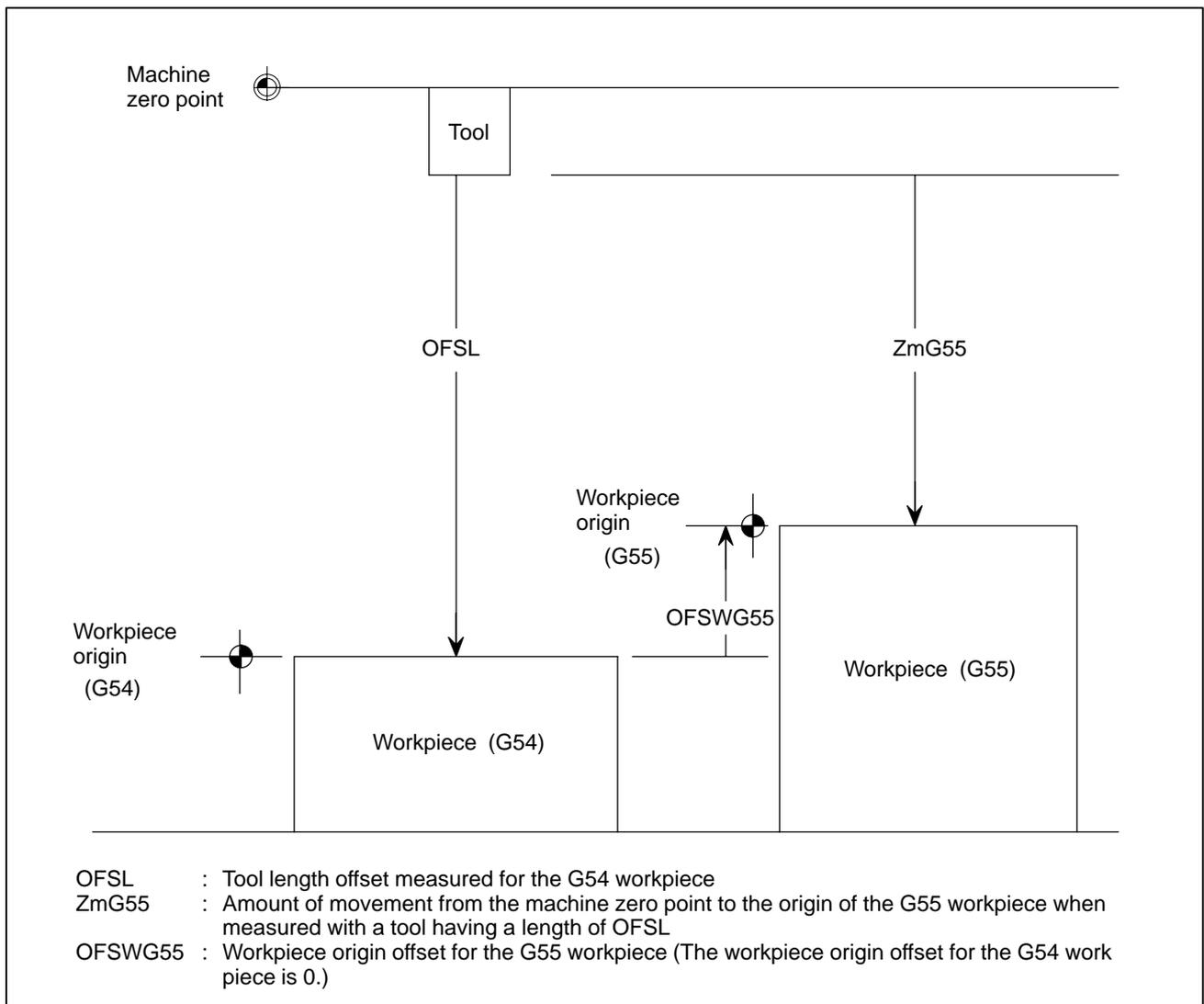
For definition 2, the workpiece origin offset can be calculated using the same formula as that used for definition 1:
