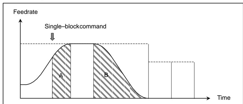
A: Amount of travel to a point where the target feedrate is attained and the current acceleration/deceleration ends
