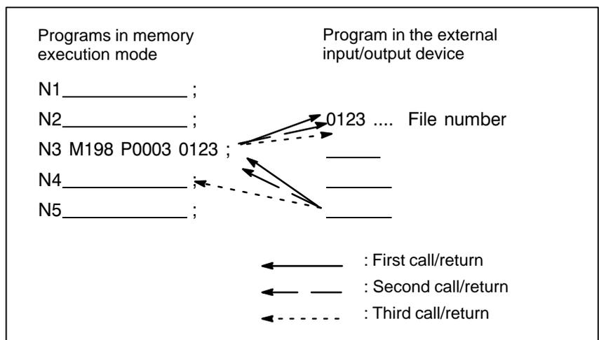
Fig. 4.7 (a) Program Flow When M198 is Specified
