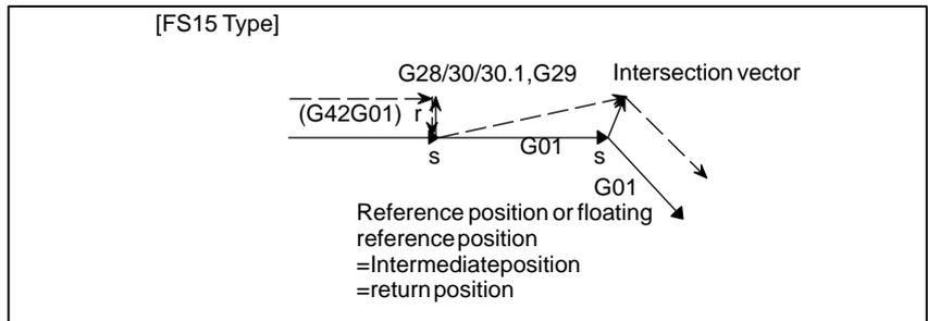
(b) For specification made other than immediately after automatic reference position return
