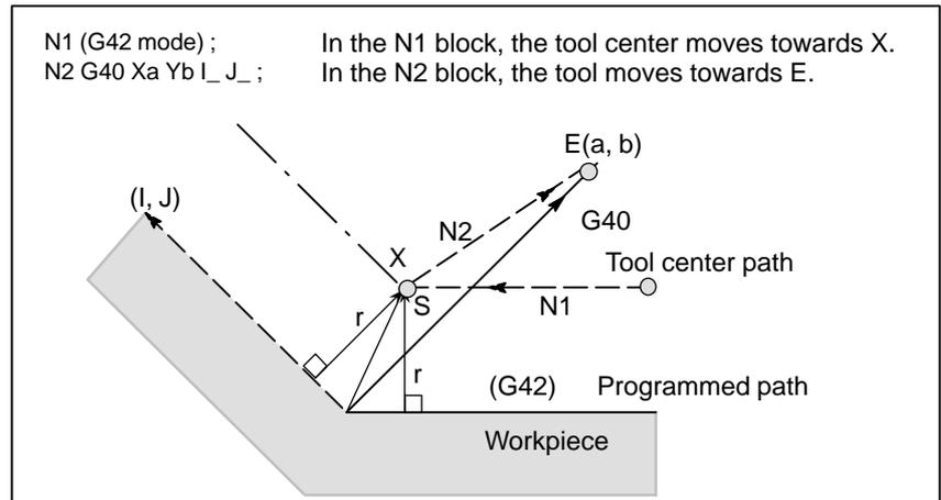
In this case, note that the CNC obtains an intersection of the tool path irrespective of whether inner or outer side machining is specified
