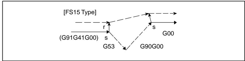
(3) G53 specified in offset mode with no movement specified
