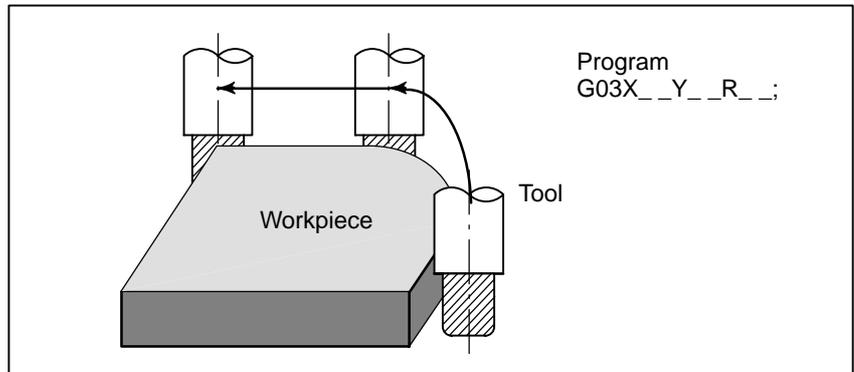
Fig. 1.1 (b) Tool movement along an arc
