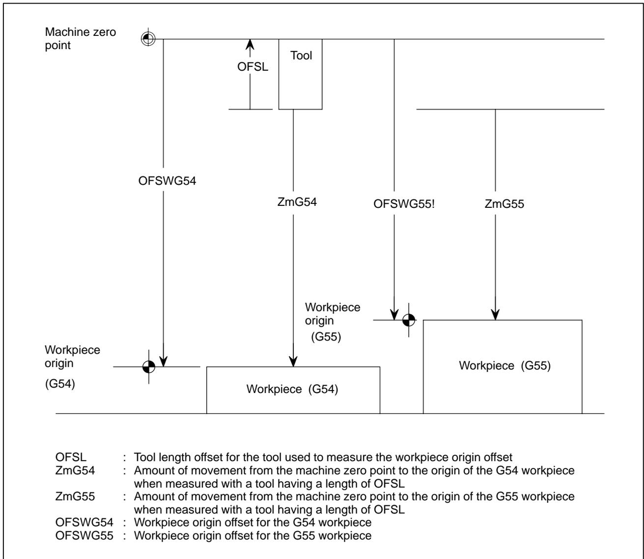
As can be seen from the above figure, the Z-axis workpiece origin offset can be calculated from the following formula:
