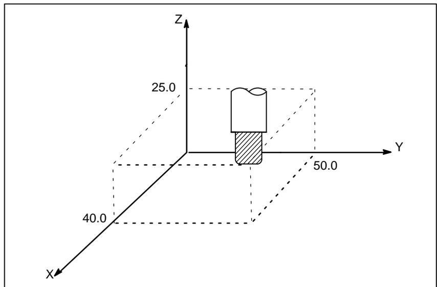
**Fig. 7 Tool Position Specified by X40.0Y50.0Z25.0**
