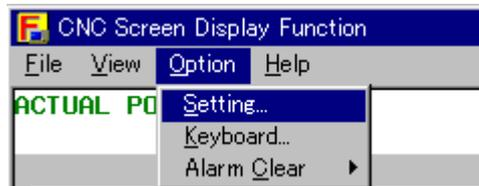
2. The Setting screen appears. Select [Lathe animation]. Set the display speed of animated simulation for turning, then choose the <OK> button.
