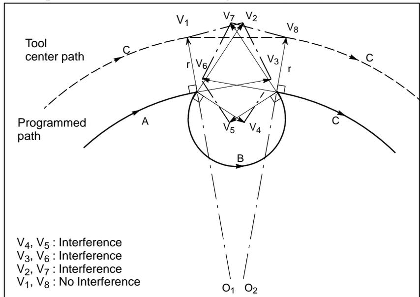
**(Example 2) The tool moves linearly from  $V_1, V_2, V_7$ , to  $V_8$**
