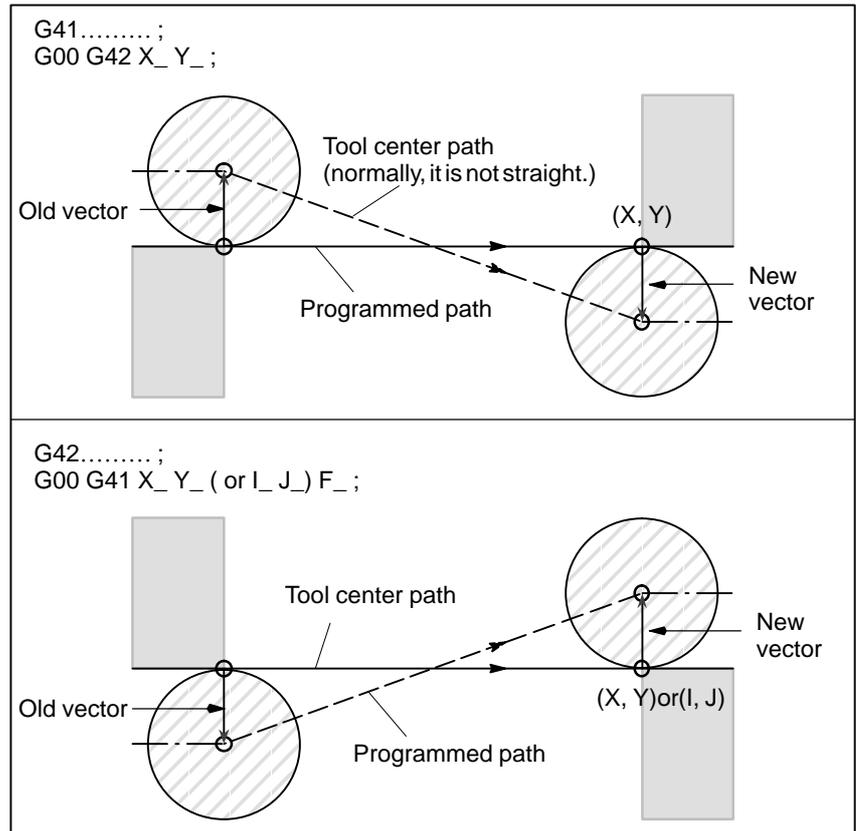
Fig. 14.4.5 Switching the Direction of Cutter Compensation
