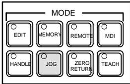
In the jog mode, pressing a feed axis and direction selection switch on the machine operator's panel continuously moves the tool along the selected axis in the selected direction.
