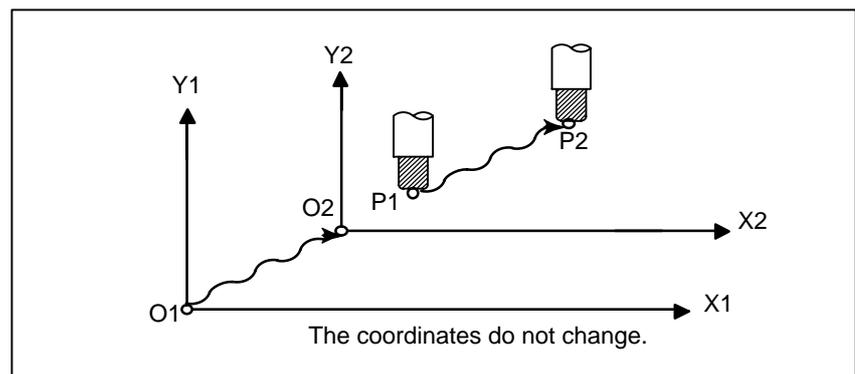
**Fig. 3.5 (b) Coordinates with the switch OFF**
