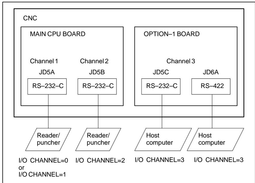
This CNC has a total of three channels of reader/puncher and remote buffer interfaces. It also has a memory card interface. The input/output device to be used is specified by setting the channel (interface) connected to that device in setting parameter I/O CHANNEL.
