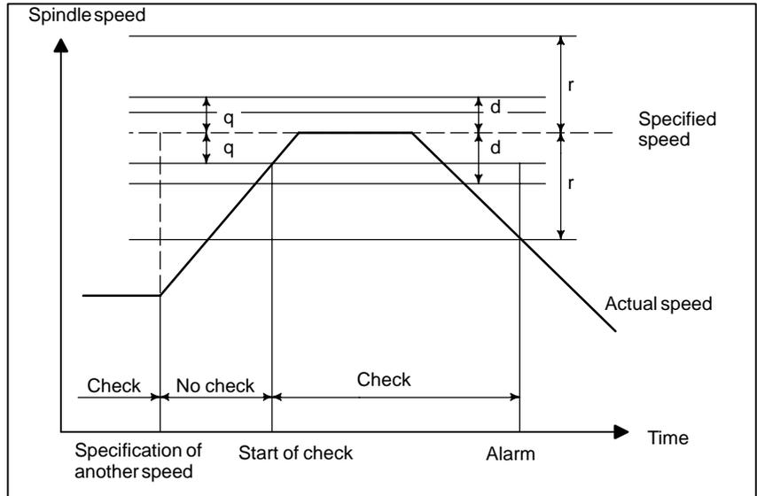
**2. When an alarm is issued before a specified spindle speed is reached**
