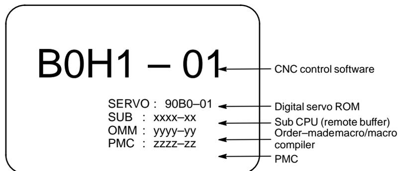
The software configuration can be displayed on the system configuration screen also.
