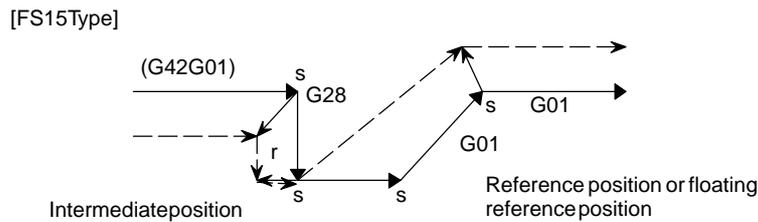
2 When G28, G30, or G30.1 is specified for a compensation axis in cutter compensation mode, the vectors along the other axes are also canceled. (This also applies when CCN (bit 2 of parameter No. 5003) is set to 1. When the FS15 type is used, only the vector along a specified axis is canceled. Note that the FS15 type cancellation differs from the actual FS15 specification in this point.)
