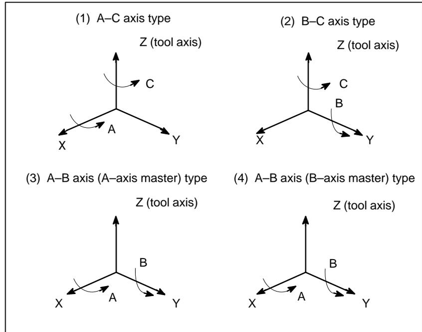
• **Pulse distribution to basic axes**
