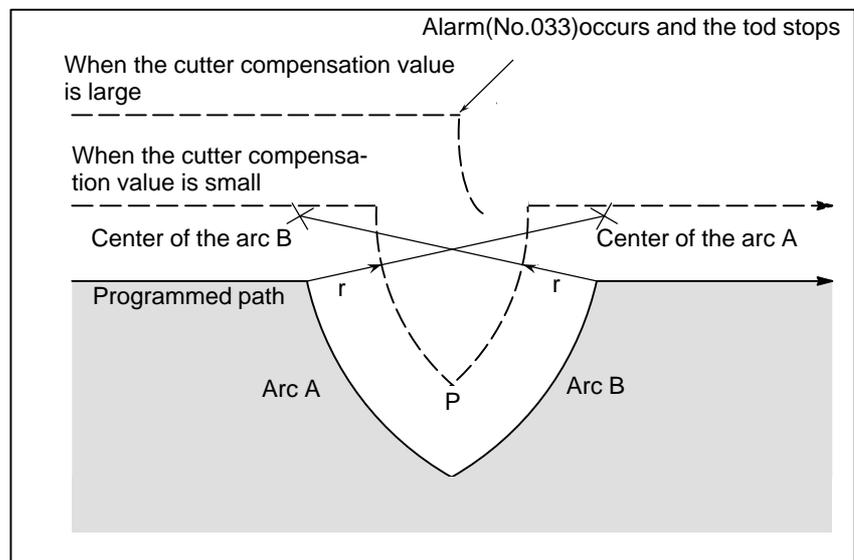
**The center of the arc is identical with the start position or the end position**
