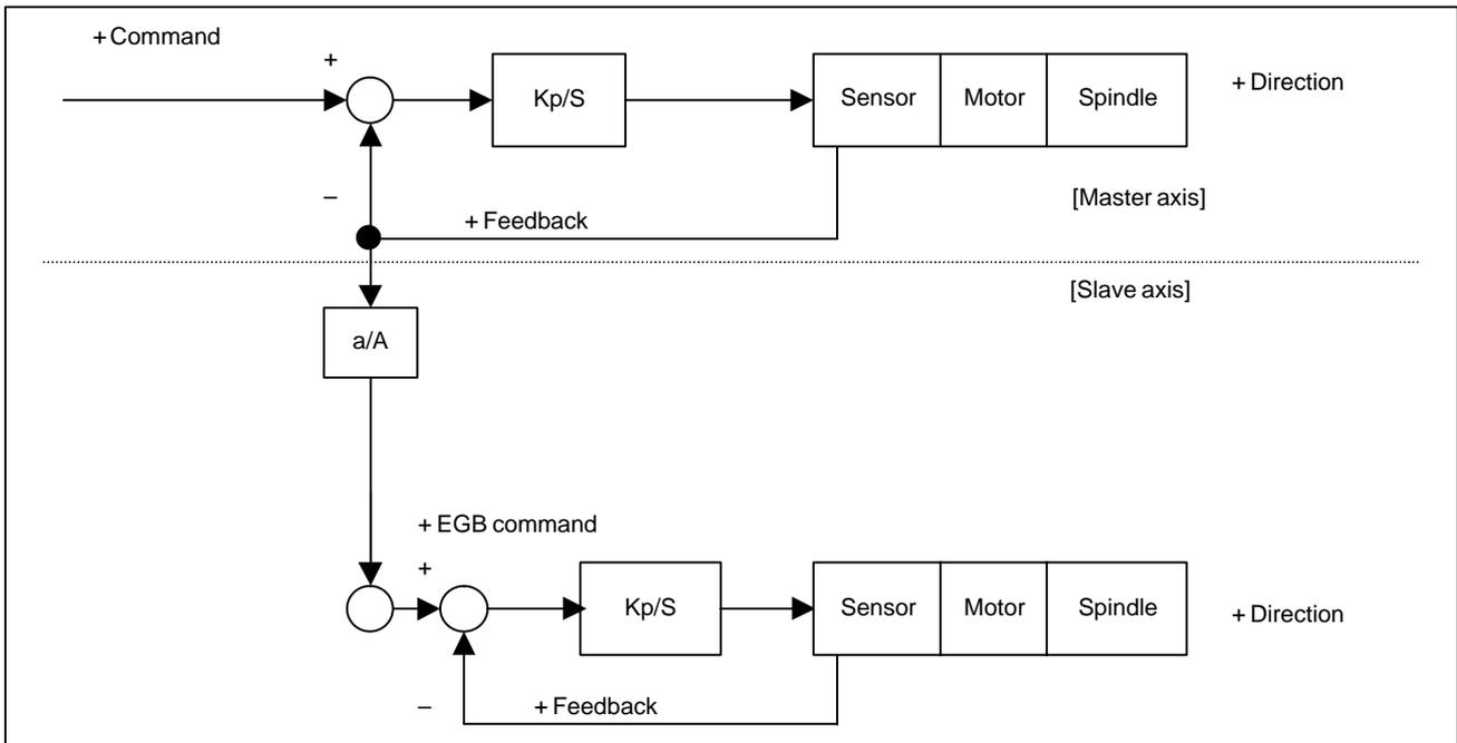
When this function is used, the SFR/SRV function in Cs contouring mode (\*) can not use. If you want to change the rotary direction of the master axis, you should change the sign of the master axis command.
