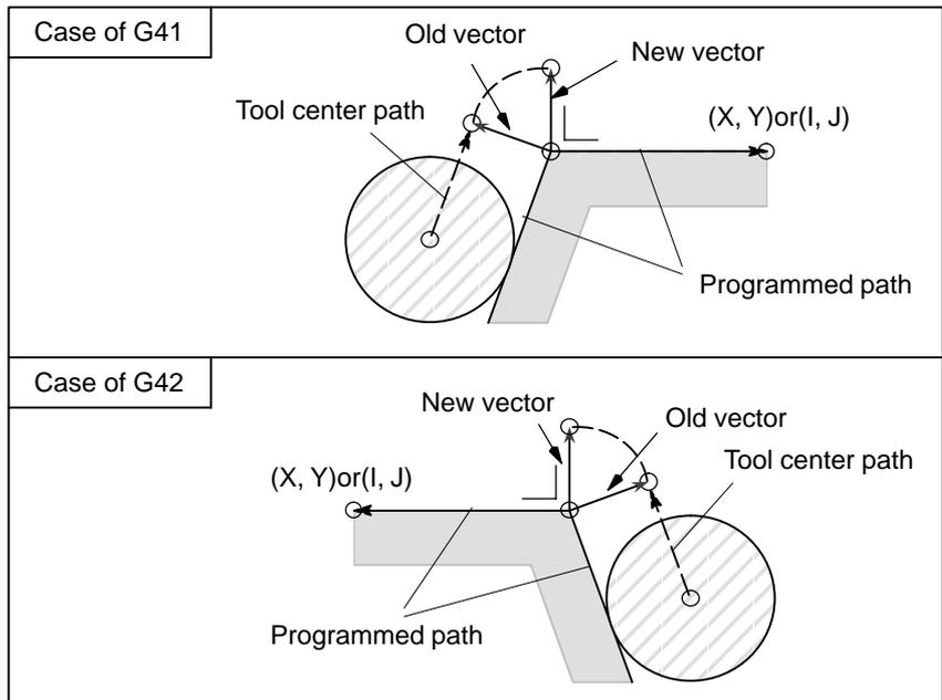
This command can be given in offset mode, that is, only when G41 or G42 has already been specified. Whether the arc is to turn clockwise or counterclockwise, is defined by G41 or G42, respectively. This command is not modal, and executes circular interpolation, whatever the G function of group 01 may be. The G function of group 01 remains even though this command is specified.
