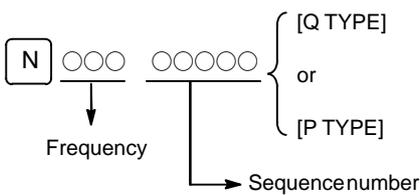
If the same sequence number appears more than once, the location of the target block must be specified. Specify a frequency and a sequence number.
