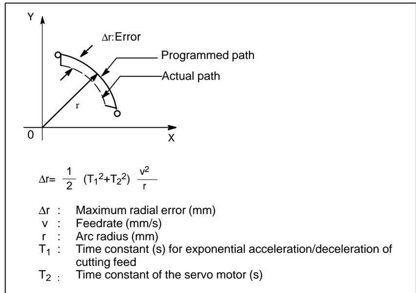
When actual machining is performed, radius  $r$  of the arc to be machined and permissible error  $D_r$  are given. Then, maximum allowable feedrate  $v$  (mm/min) is determined from the above expression.
