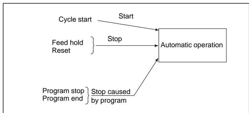
**Fig. 1.3 (b) Start and Stop for Automatic Operation**
