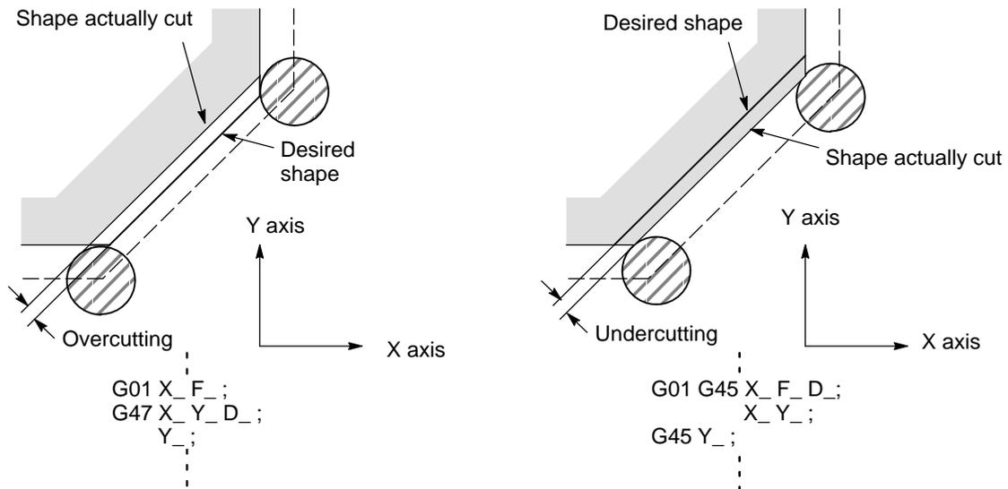
2 G45 to G48 (tool offset) must not be used in the G41 or G42 (cutter compensation) mode.
