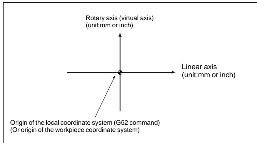
**Fig. 4.8 (a) Polar coordinate interpolation plane.**
