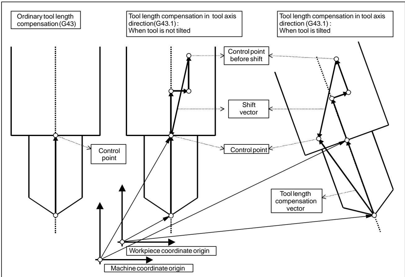
Fig. 22.4 (e) Shift of the Control Point
