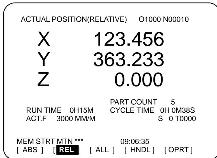
The number of machined parts (PART COUNT), run time (RUN TIME), and cycle time (CYCLE TIME) are displayed under the current position.
