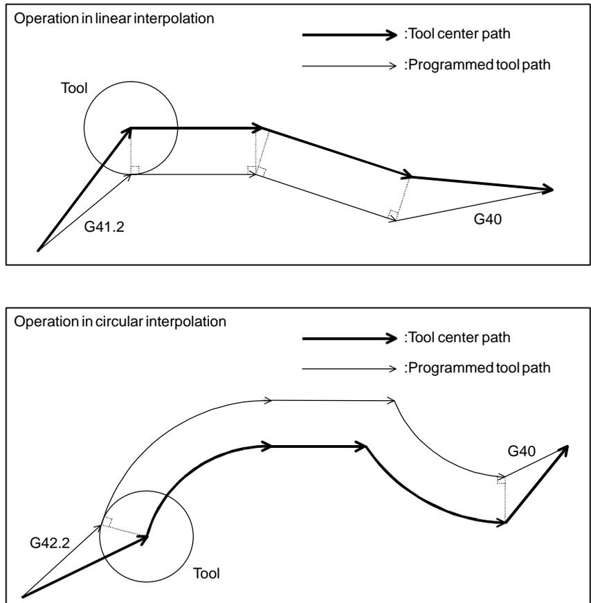
**Fig. 22.5.1 (b) Operation at compensation start-up and cancellation (Type A)**
