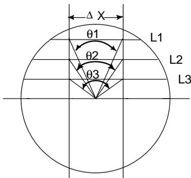
Consider lines L1, L2, and L3.  $\Delta X$  is the distance the tool moves per time unit at the feedrate specified with address F in the Cartesian coordinate system. As the tool moves from L1 to L2 to L3, the angle at which the tool moves per time unit corresponding to  $\Delta X$  in the Cartesian coordinate system increases from  $\theta_1$  to  $\theta_2$  to  $\theta_3$ .
