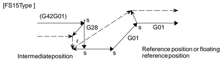
Example2: When CCN (bit 2 of parameter No.5003)=1 and each-axis machine lock is applied
