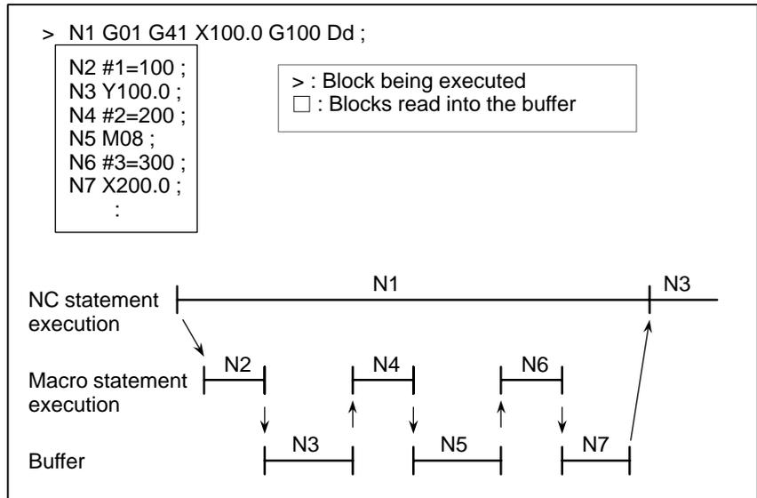
When the N1 is being executed, the NC statements in the next two blocks (up to N5) are read into the buffer. Since N5 is a block that involves no movement, an intersection cannot be calculated. In this case, the NC statements in the next three blocks (up to N7) are read. The macro statements (N2, N4, and N6) between N1 and N7 are processed during execution of N1.
