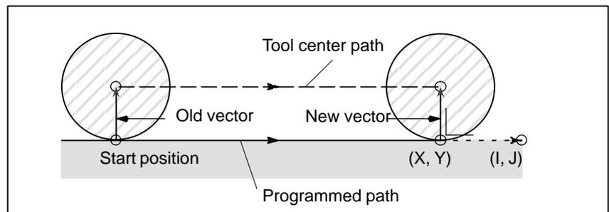
In case the old vector is 0, this command specifies the equipment to enter from the cancel mode into the cutter compensation mode. At this time, the offset number is specified by the H code.
