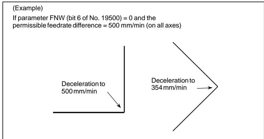
If "1" is set, the feedrate is determined not only with the condition that the permissible feedrate difference and permissible acceleration on each axis are not exceeded, but also that the deceleration feedrate is constant regardless of the travel direction if the shape is the same.
