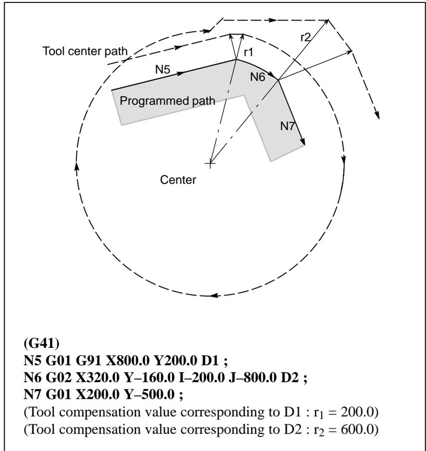
In the above example, the arc in block N6 is placed in the one quadrant. But after cutter compensation, the arc is placed in the four quadrants.
