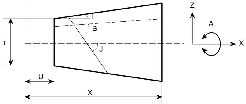
**Constant helix machining for producing a reverse tapered figure**
