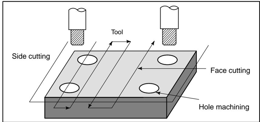
Prepare the program of the tool path and machining condition according to the workpiece figure, for each machining.
