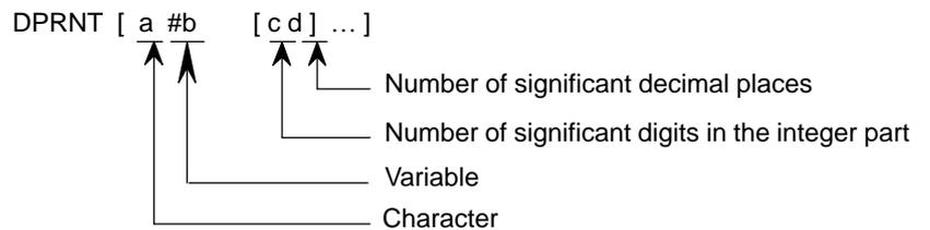
The DPRNT command outputs characters and each digit in the value of a variable according to the code set in the settings (ISO).
