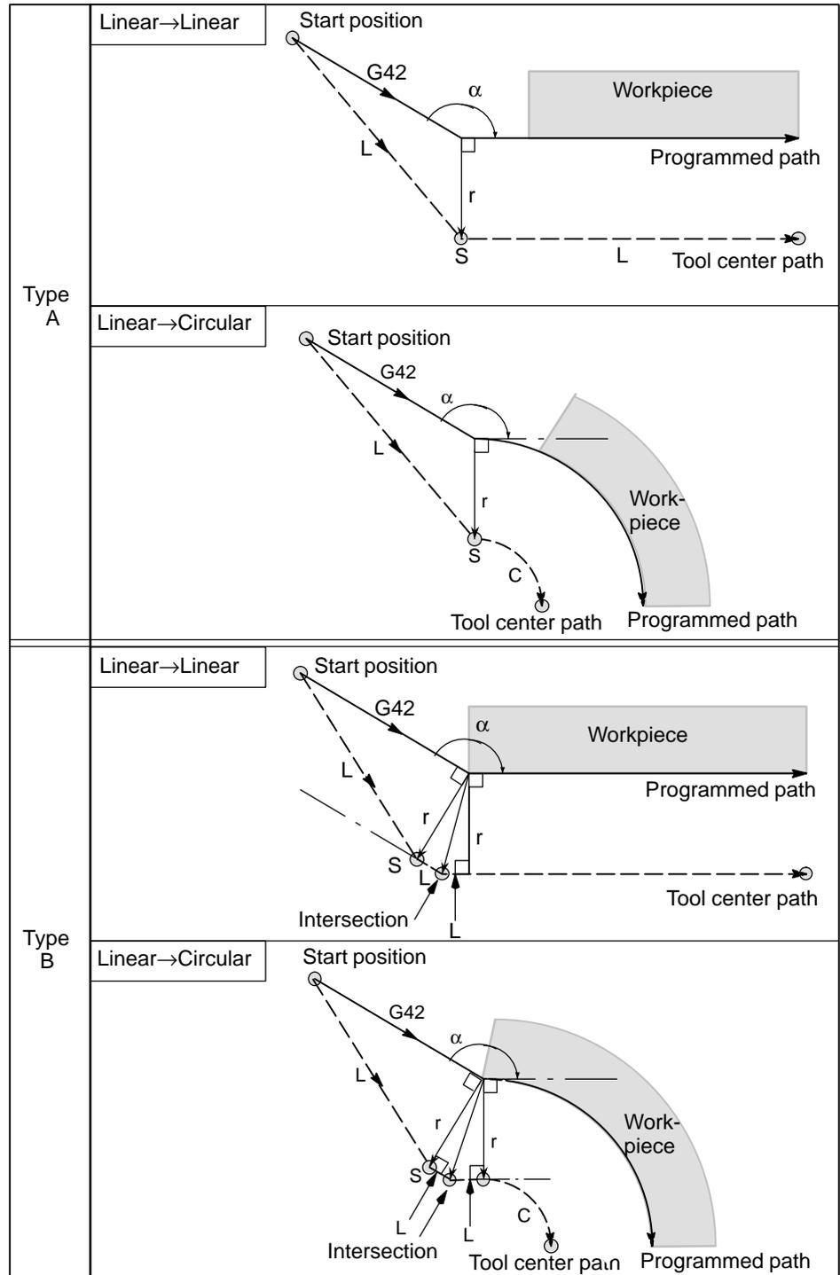
● **Tool movement around the outside of an acute angle ( $\alpha < 90^\circ$ )**
