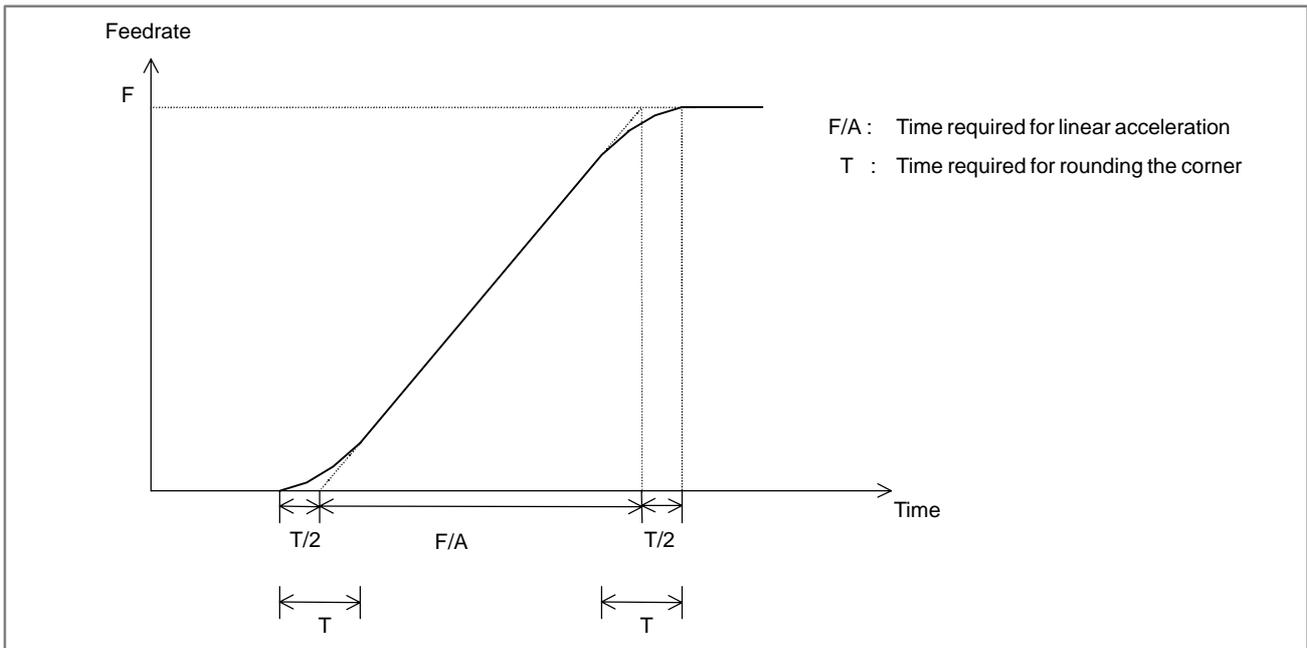
When the non-linear interpolation type is selected, movement is performed at the feedrate set in parameter No. 1420 with acceleration/deceleration set in parameter No. 1620. The corresponding value can be set in parameter No. 1621 to select bell-shaped acceleration/deceleration. (To select bell-shaped acceleration/deceleration, the option of bell-shaped acceleration/deceleration for rapid traverse is required.)
