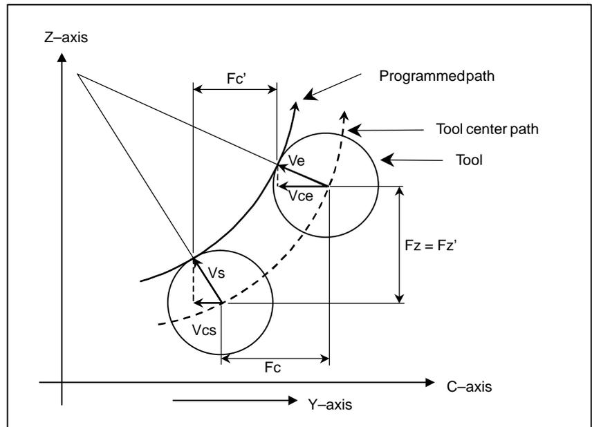
Fig. 22.2 (h) Actual Speed Indication during Circular Interpolation
