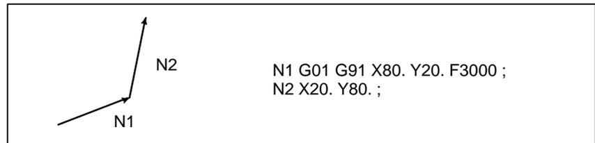
When this movement is specified, the feedrate along each axis is as shown in the next figure.
