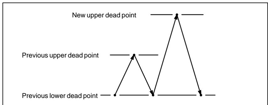
The tool first moves to the previous upper dead point, then to the lower dead point, and finally to the new upper dead point.
