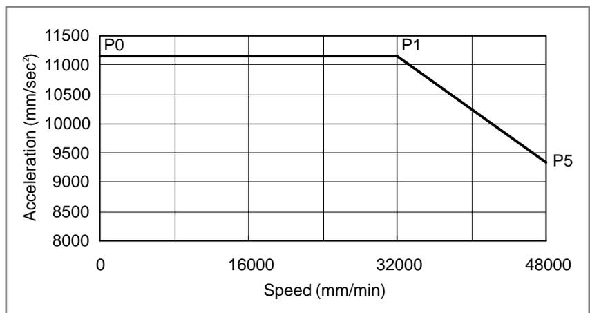
Fig.19.10(j) Acceleration pattern in case of + move and deceleration
