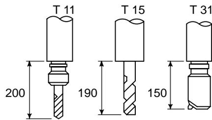
Offset value +200.0 is set in offset No.11, +190.0 is set in offset No.15, and +150.0 is set in offset No.31
