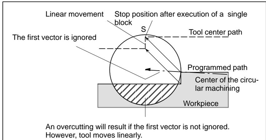
● **Starting compensation and cutting along the Z-axis**
