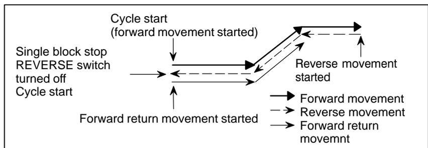
In the case of 3) above, the tool starts forward return movement at the position of a feed hold stop when the cycle start switch is pressed.
