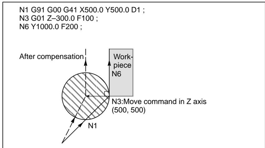
In the program example above, when executing block N1, blocks N3 and N6 are also entered into the buffer storage, and by the relationship among them the correct compensation is performed as in the figure above.
