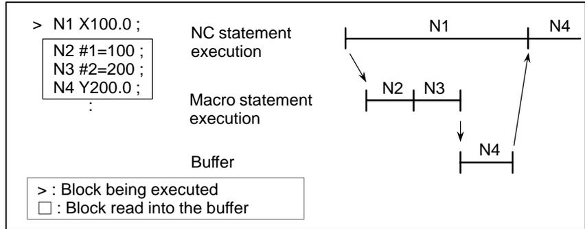
When N1 is being executed, the next NC statement (N4) is read into the buffer. The macro statements (N2, N3) between N1 and N4 are processed during execution of N1.
