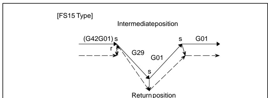
(3) G29 specified in offset mode (with movement to a reference position not performed)
