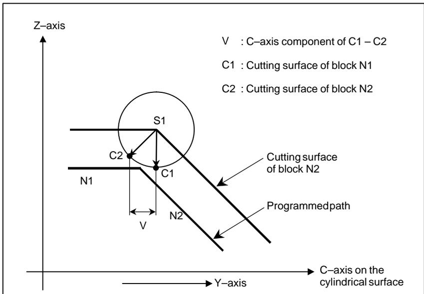
**Fig. 22.2 (b) Cutting Point Compensation between Blocks**
