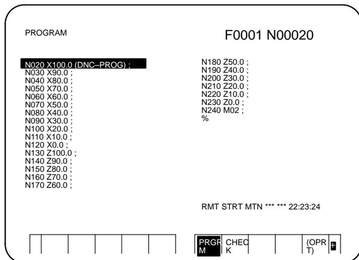
During DNC operation, the program currently being executed is displayed on the program check screen and program screen.
