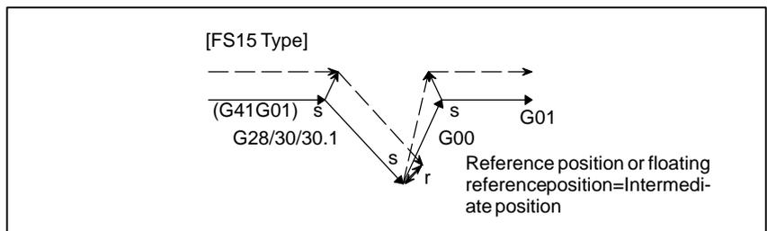
(4) G28, G30, or G30.1 specified in offset mode (with no movement performed)
