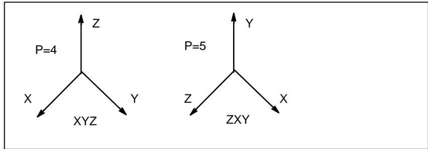
Fig. 12.2.1 (a) Coordinate systems for the isometric projection
