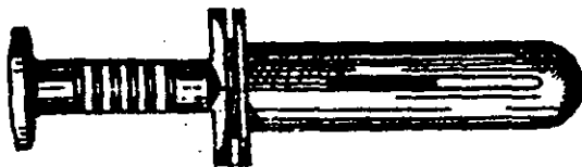
FIGURE 19.—Shield, expansion, nail anchor (aluminum).
