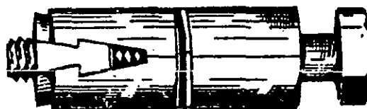
FIGURE 11.—Shield, expansion, anchor (machine bolt). Style 1. Single-end expansion shield anchor.
