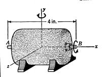
The rotor of an electric motor weighs 6 lb and has a radius of gyration of 2 in. The angular velocity of the rotor is 3,600 rpm counterclockwise as viewed from the positive x axis. Determine the reactions exerted by the bearings on the axle AB when the motor is rotated about the y axis clockwise as viewed from above and at a rate of 6 rpm.
