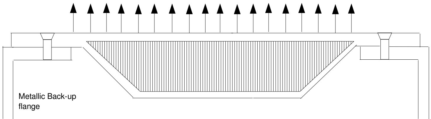
Heel & Toe Force and Fastener Reaction
