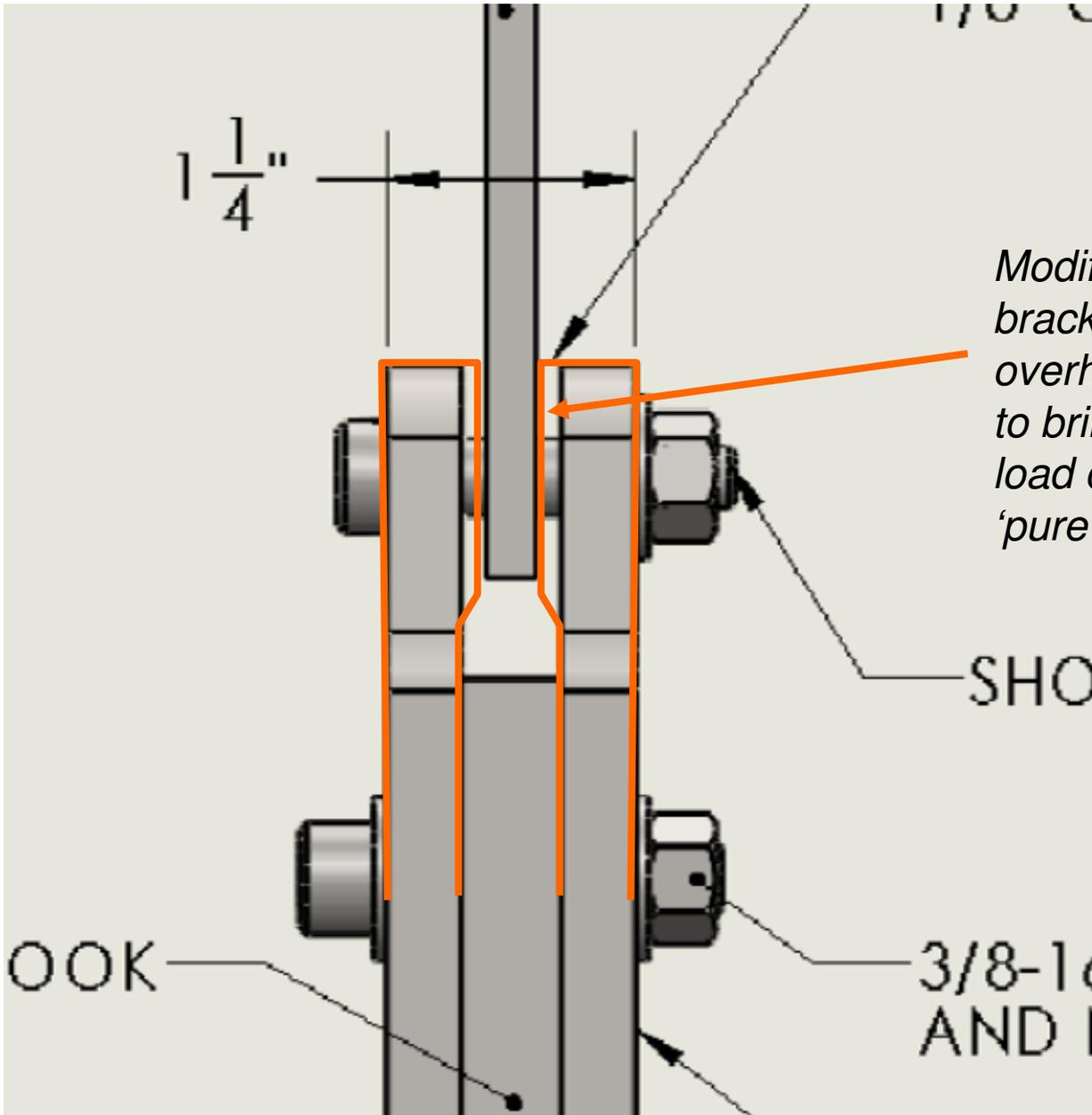
*Modify the hook brackets to overhang slightly, to bring the pin load closer to a 'pure shear' case.*
