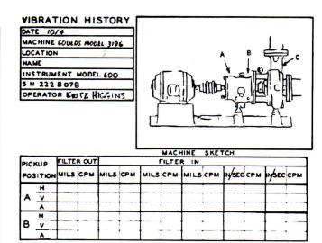
Fig. 4 Vibration Data Sheet
