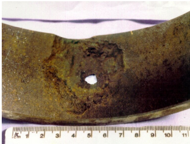
Figure 9 Pitting in a Sour System
