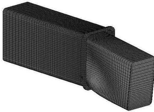
Fig. 3: Simplified model of part of a telescope crane at the onset of buckling
