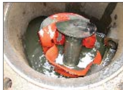
Lost pig found in check valve at valve station 1.
