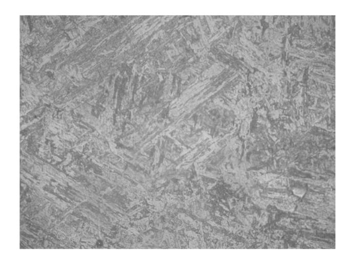
Photomicrograph 1: Coarse grain tempered martensite. Hardness 225 Hv. As supplied microstructure for T91, normalize and tempered. Microstructure is almost similar to weld metal in welding.
