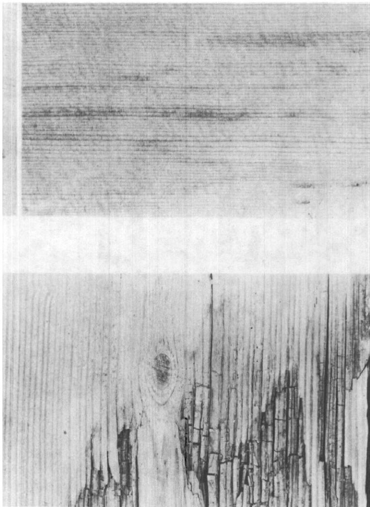
Figure 2-2. Stages of decay. (Top) Early stage evidenced by discoloration in surface and, at left, in end grain. (Bottom) Late stage, with cracked and collapsed wood. An abnormal brown color will be imparted to the wood by this type of decay.
