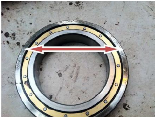
Drive End bearing outer runner axially Damaged
