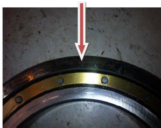
Drive End bearing outer runner axially Damaged
