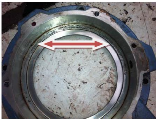
Outer Bearing Housing Damaged
