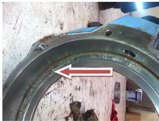
Outer Bearing Housing Damaged
