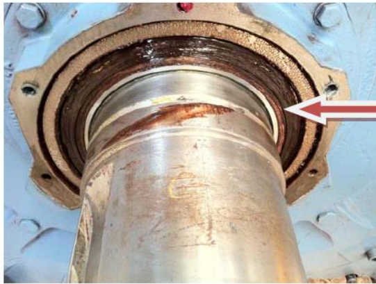
Bearing grease Decolorised
