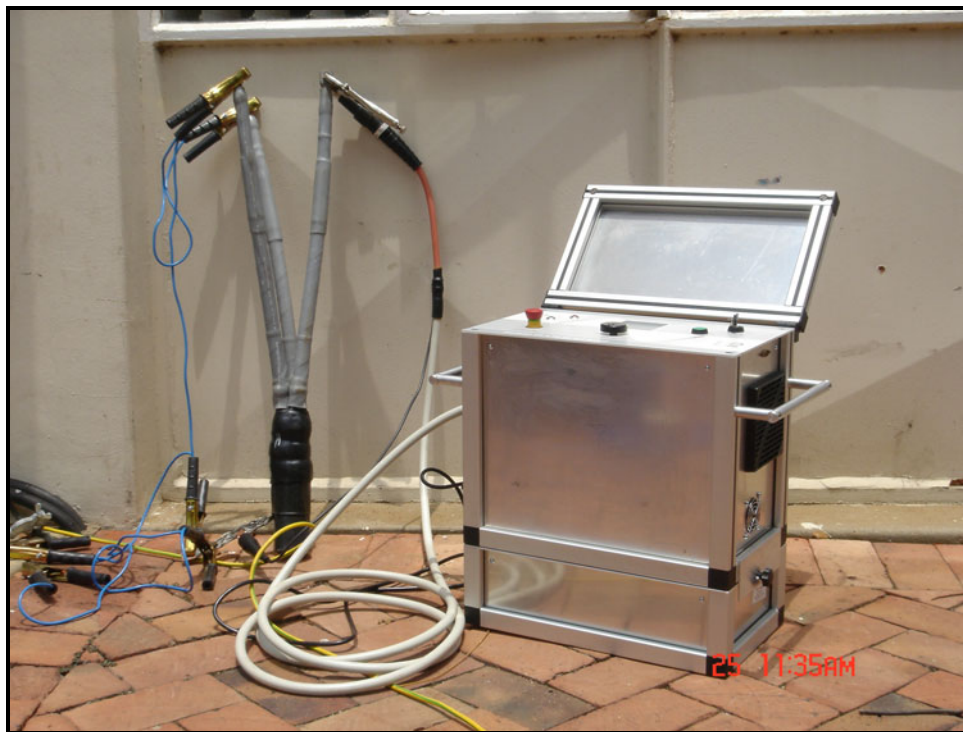
Figure 5: A typical connection setup for a VLF cable test. Note the grounding of the other two phases, while the third phase is being tested.
