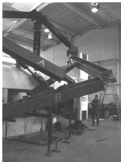
Test set-up for full-scale seismic loading of a precast concrete, hollow core diaphragm and its related concrete structural components at the University of Canterbury, 2003.
