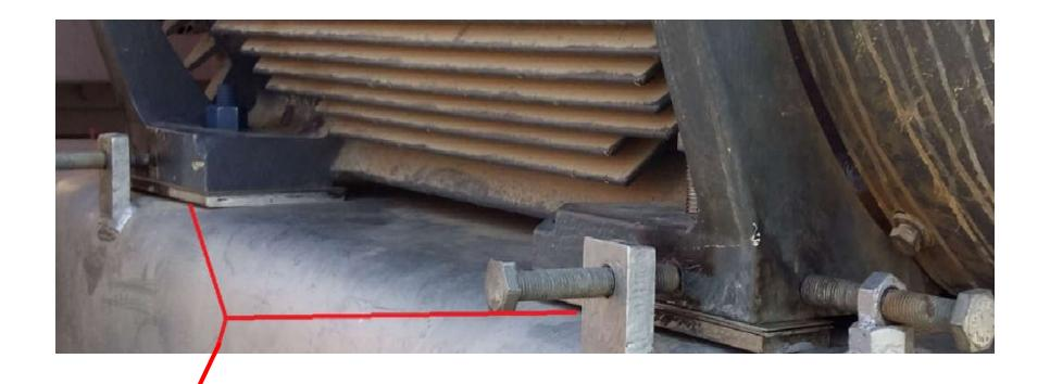
Is welding of pad to the mounting base to assist in elimination of soft foot is an acceptable solution
