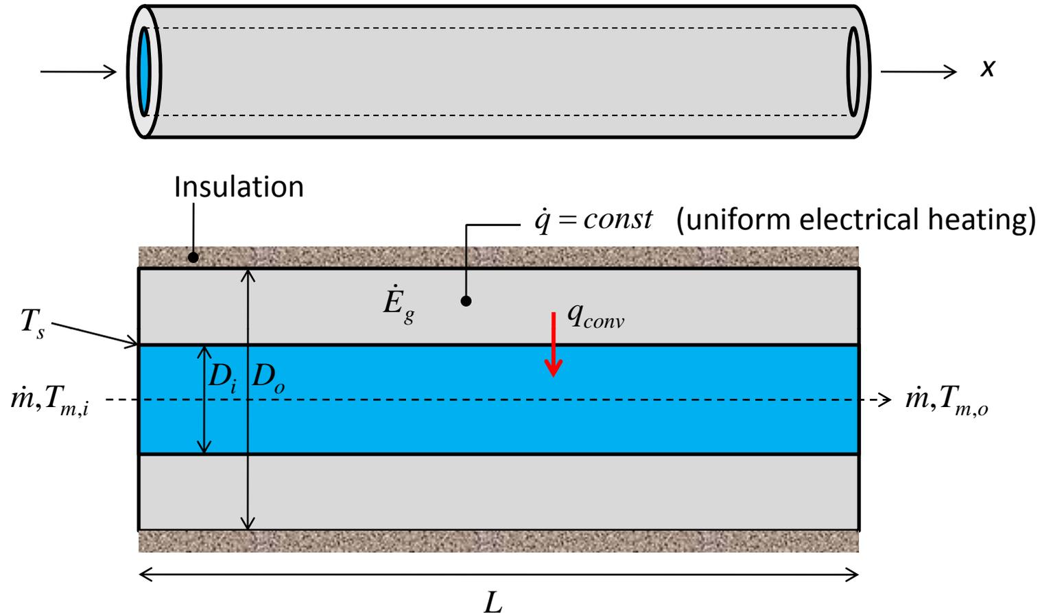
**Known:** Internal flow through thick-walled tube having uniform heat generation.
