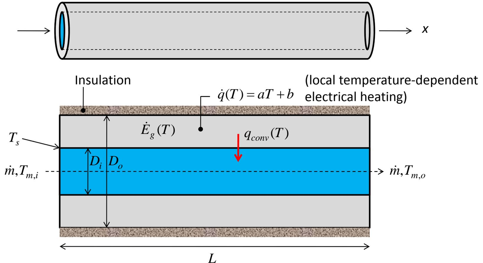
**Known:** Internal flow through thick-walled tube having NON-uniform heat generation.
