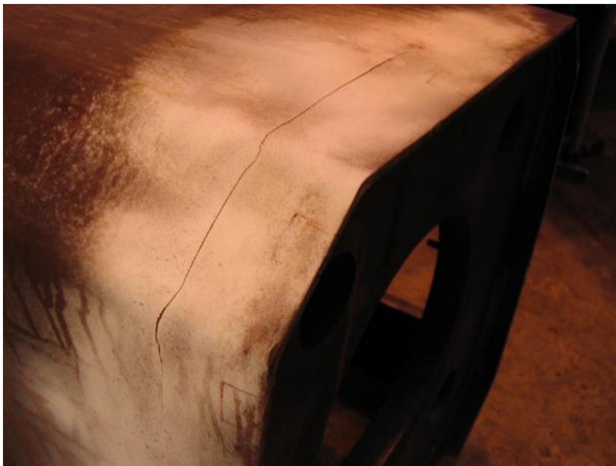
Figure 7.26 Crack in second transformer base.
