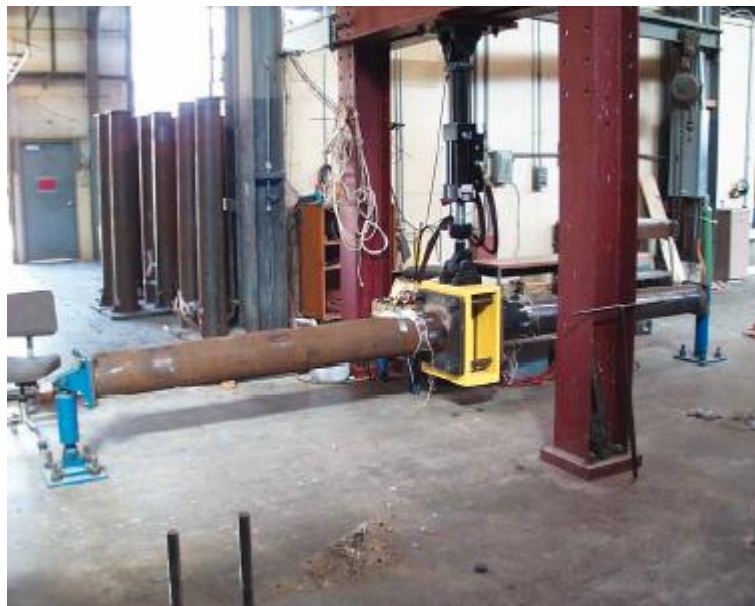
Figure 3.22 UTexas mast arm fatigue setup.
