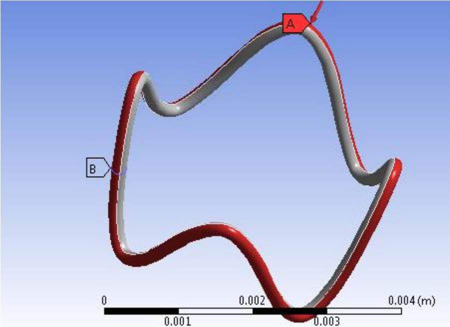
In the next figure shown below, the shadowy ring shows the original undeformed, fully expanded stent ring. The brighter, more prominent shape represents the stent half-way thru its squeezed shape.
