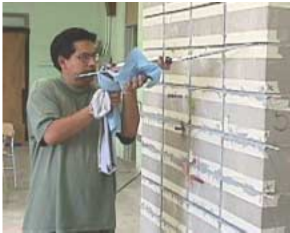
(a) Application of Embedding Paste
