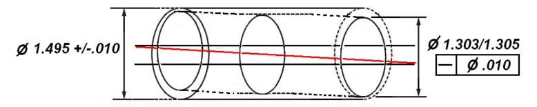
Wall thickness can be as thin as .085 ((1.485 - 1.315)/2) or As thick as .106 ((1.505 - 1.293)/2) ?
