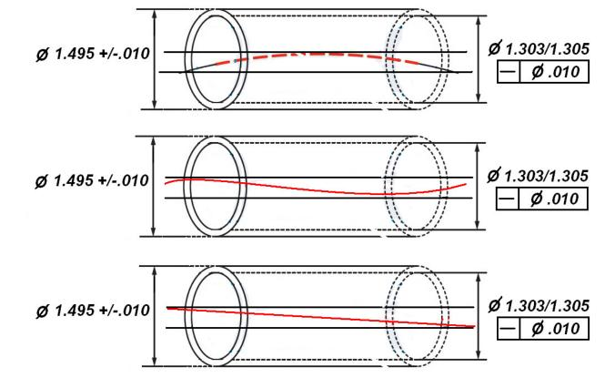
Straightness is only called out for the inner Diameter.
