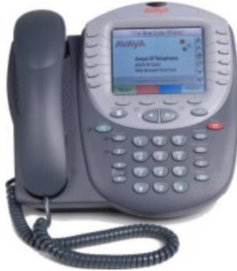
IP Office release 3.2 will also introduce support for the 4625SW IP telephone. The 4625SW supports access to the World Wide Web as well as offering the latest features and applications. The large display area allows up to 12 application-specific buttons to be presented and labelled. Additionally, 12 Line/Feature buttons, 4 soft keys, and other fixed buttons provide access to powerful capacities such as:
