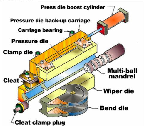
die will travel with the tube as it is being formed. The pressure die boost cylinder is attached to the pressure die. The boost cylinder can assist the tube through the bend to prevent tube breakage, wall thinning and ovality.
