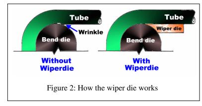
The wiper die is made so that it can nest in the bend die groove with its very thin tip extending to the bend tangent point (the point where the tube will begin to bend). In doing so, it fills up the gap normally left by the bend die. Therefore, the tube is completely confined and does not have space in which to wrinkle.
