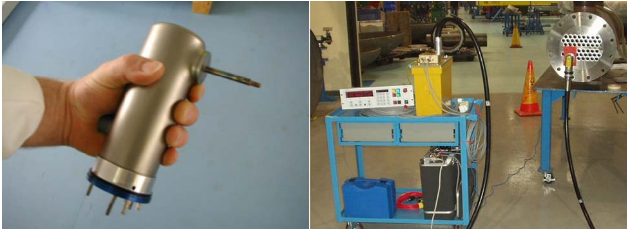
Figure 3. Rod anode X-ray tube MCTS 130-0.6 (left side) and complete inspection setup with controller (right side): HV generator [2] and X-ray tube with film holder (red) at a heat exchanger ready for single-sided inspection
