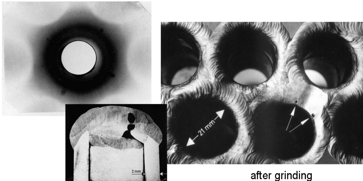
Figure 2. Film exposure (left above) and corresponding cross sections by destructive testing (left down and right) showing typical flaws like porosities and notches
