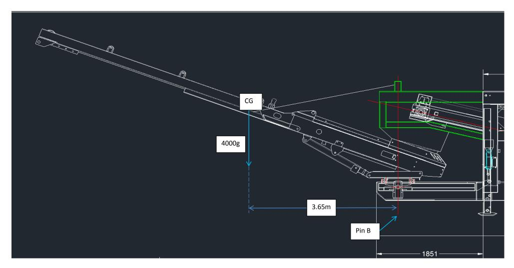
The linkage will be acting about the pin B as indicated, to turn the table which rotates about the same axis. The conveyor is then attached to this turn table. Lets take for now that the 4000kg mass acts through the centre of gravity CG at 3.65m from the axis of rotation. (just assume mass of turntable is negligible for now)
