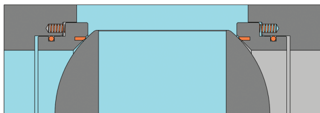
Uni-directional seat Self relieving condition
