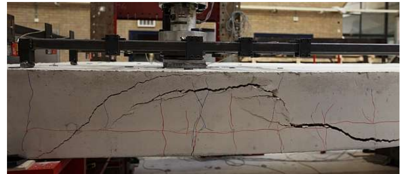
Punching shear, two-way shear
