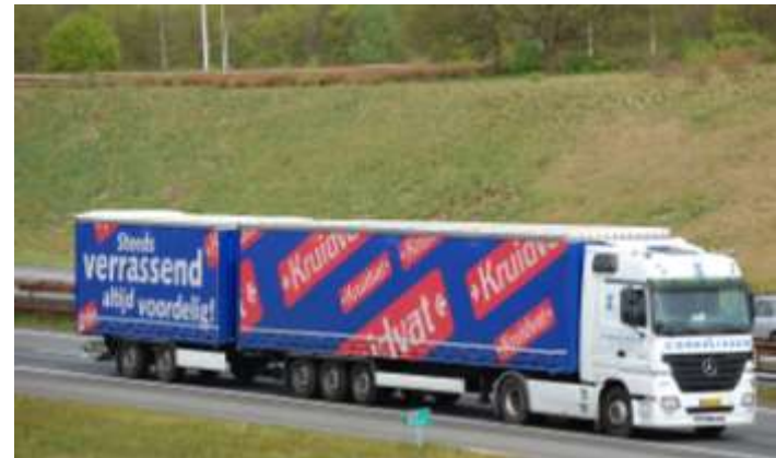
heavy and long truck (600 kN > perm. max = 50ton)
