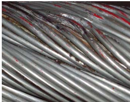
View of haul rope damage at 576 meters from splice
