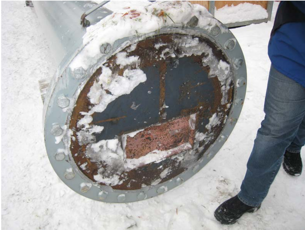
Lower Excalibur T4, underside of lower section cap plate, shiny weld surface shows brittle plate failure (i.e. plate tore away from the weld)
