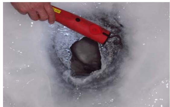
Partially Frozen Ice Column Inside Tower #4 Lower Section Tube
