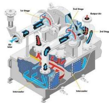
this point, the compressor is unable to maintain a steady flow of air into the system. When this point is reached, backflow from the system through the compressor occurs until a momentary equilibrium is established between the compressor and the system.
