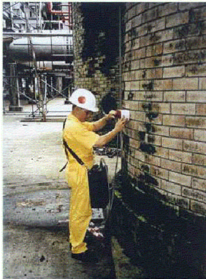
Pulsed Eddy Current inspection of a steel skirt through fire-proofing
