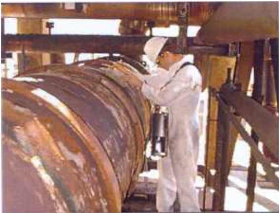
In-service inspection of a heat exchanger at high temperature. Several readings are taken along the circumference of the shell
