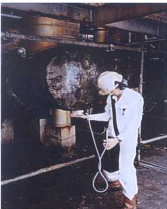
Inspection of a shell of an insulated heat exchanger
