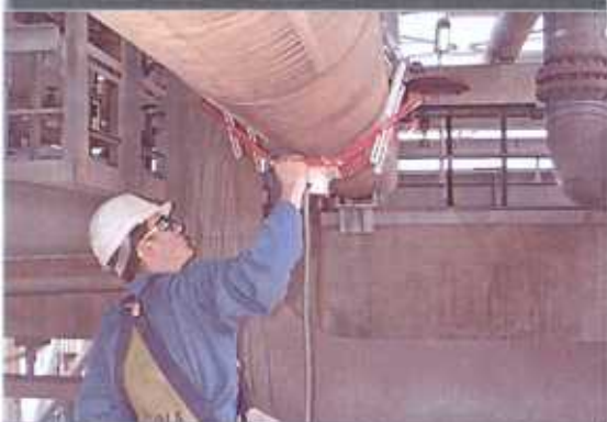
Inspection of an insulated line Several readings are taken along the bottom of the pipe
