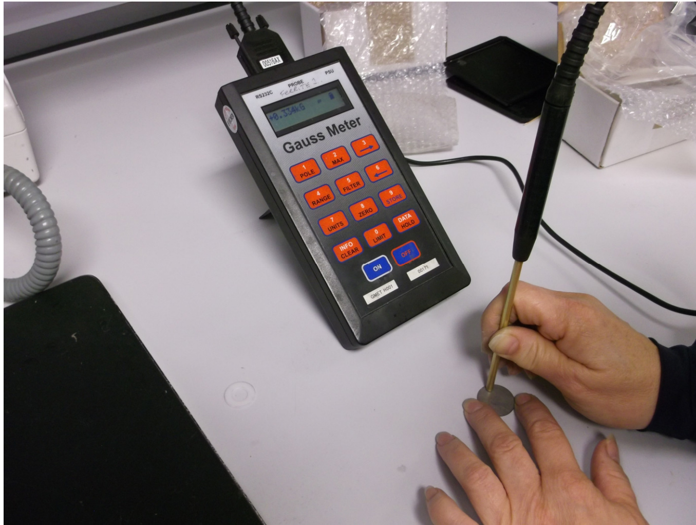
Test Setup :- Gauss Meter PRF 458. Magnets probed at centre, near edge at 3 o'clock, near edge at 6 o'clock, near edge at 9 o'clock, near edge at 12 o'clock
