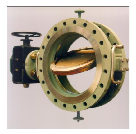
Vanessa recommends the installation of the jacketed valves with the shaft horizontal (see figure 1 and figure 2) in order to prevent any possible fluid deposit into the lower bearing areas, and to avoid the increasing of the operational torque.
