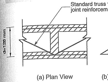
**Figure 6.26** Reinforced masonry wall joint reinforcement.
