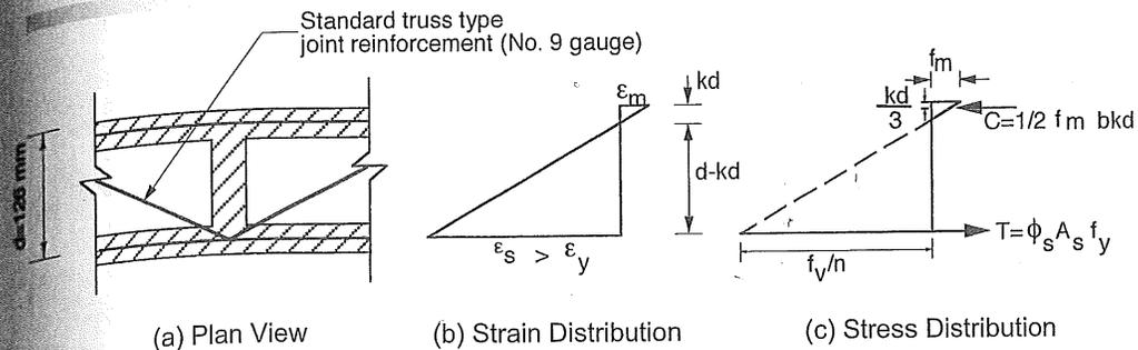
Figure 6.26 Reinforced masonry wall spanning horizontally for Example 6.5.
