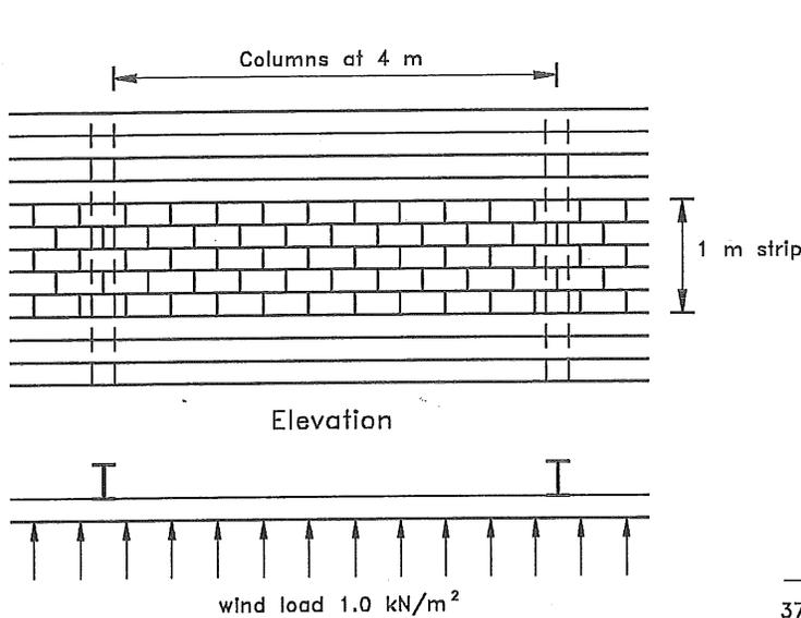
Fig. 3-8 Wall of Example 3-5
