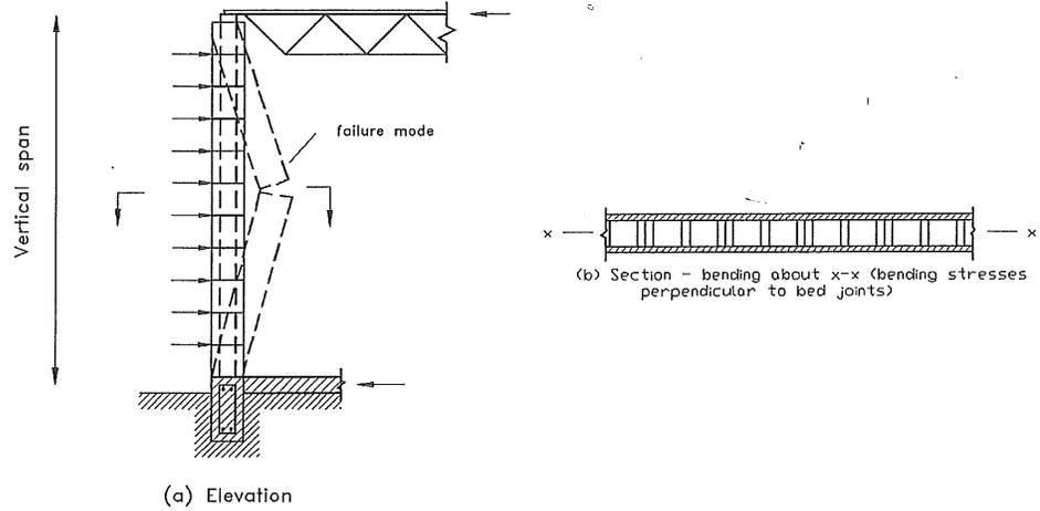
Fig. 3-6 Wall With Vertical Span
