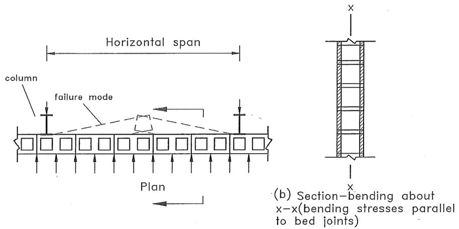
Fig. 3-7 Wall With Horizontal Span
