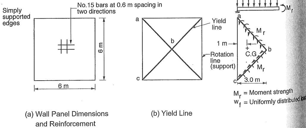
**Figure 6.25** Reinforced masonry wall under two-way bending for Example 6.4.
