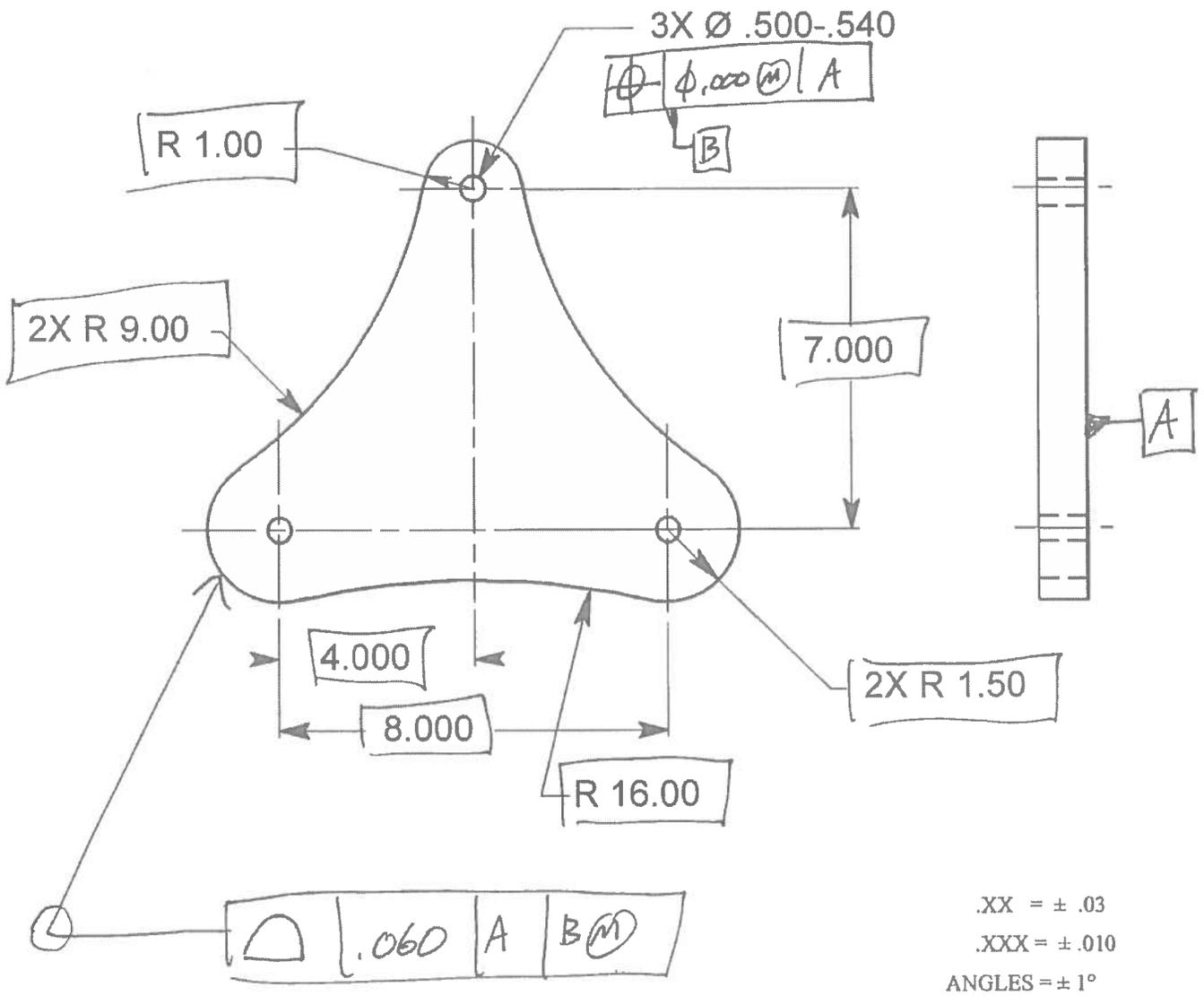
39. The hole pattern is for ½-inch fasteners. Locate the three holes to each other and perpendicular to the back of the part within the required tolerance. Next specify a profile tolerance perpendicular to the back of the part and located to the hole pattern within .060. Complete the drawing using MMC/MMB wherever possible.
