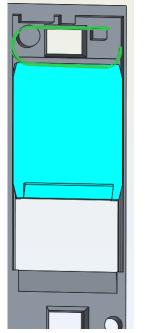
Cyan shutter is raised, bending spring as shown (in fact the top face is slightly bowed, not straight as shown here)
