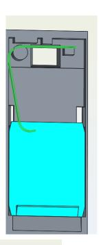
Flat spring shown in green. 1mm wide, 0.25mm thick, Galvanised spring steel.
