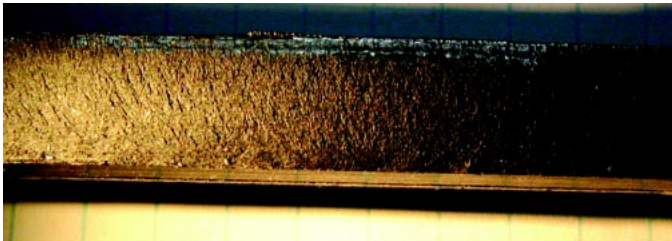
Photo 4 A view of a low-cycle fatigue failure of a gear tooth from a large compressor. Note that both the coarse ratchet marks on the left and the fine ones to the right point away from the origin, which is on the bottom edge of the tooth, just to the right of the center.
