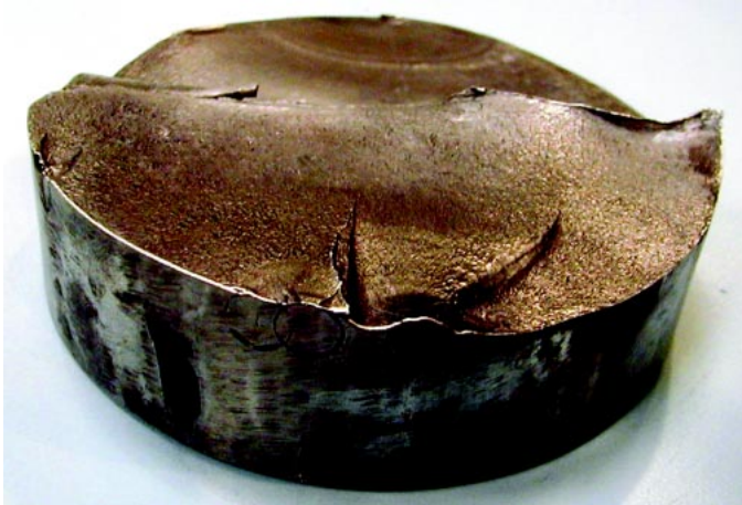
Photo 2 A view of an agitator shaft showing two ratchet marks separating the three failure origins. Note that the origins are not on the same plane and that the ratchet marks are in effect boundaries between the fracture planes. (There is yet another origin on the other side of the failure face.)
