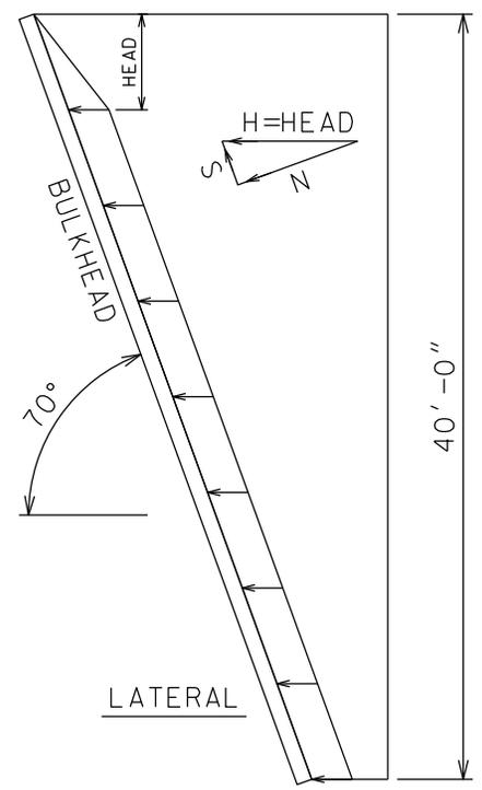
LOAD APPLIED TO BULKHEAD AS VERTICAL LINEARLY DISTRIBUTED:  $W = V * \cos 70^\circ$
