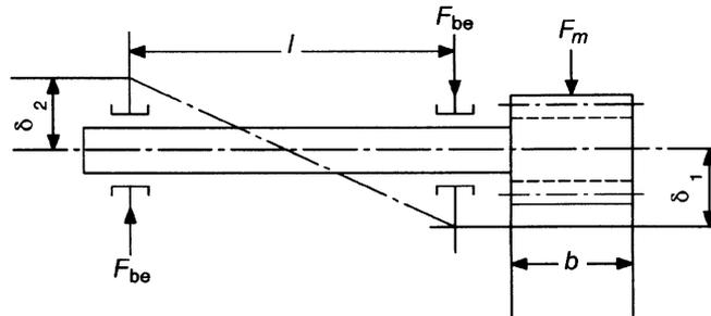
Figure 19 — Loading and deflections for an overhung gear, see equation (101)
