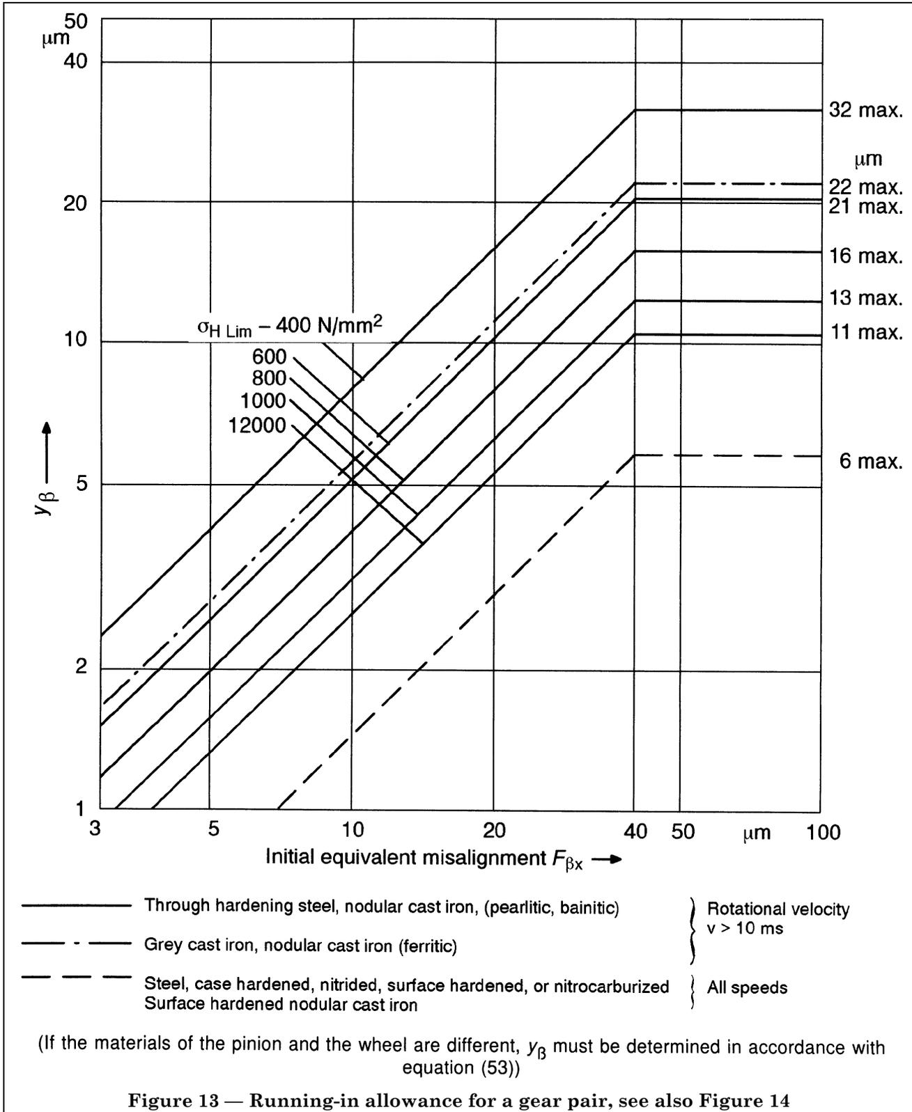
When the material of the pinion differs from that of the wheel, the values for the pinion ( $y_{\beta 1}$  and  $\chi_{\beta 1}$ ) and the values for the wheel ( $y_{\beta 2}$  and  $\chi_{\beta 2}$ ) are to be determined separately. Then the average values, of each ( $y_{\beta}$  and  $\chi_{\beta}$ ) from equations (53) and (54), are used for the calculations.
