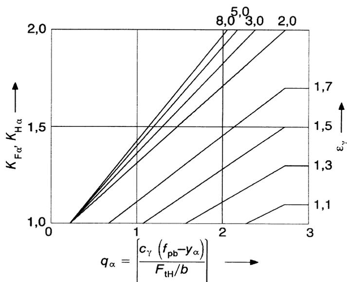
Figure 26 — Determination of the transverse load factors  $K_{H\alpha}$  and  $K_{F\alpha}$  by method B (see 8.3.3 and 8.3.4 for limiting conditions)
