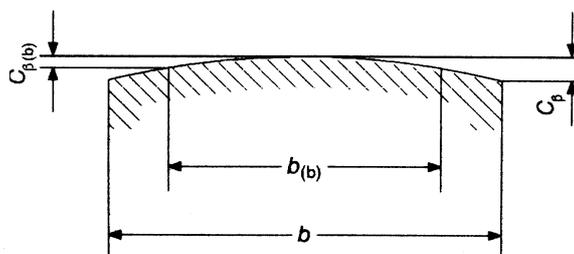
Figure A.1 — Amount of crowning  $C_{\beta(b)}$  and width  $b_{(b)}$  (see 7.6.2.2)
