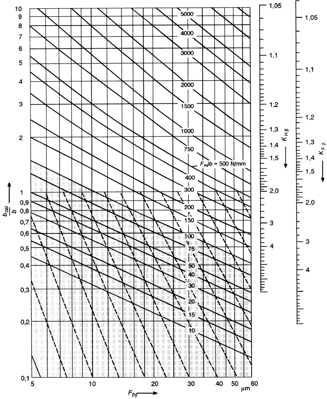
Figure 12 — Face load factors  $K_{H\beta}$  (contact stress) and  $K_{F\beta}$  (tooth-root stress) for values of  $b/h < 12$  in accordance with method C2 (simplified method in which  $c_y = 20 \text{ N}/(\text{mm } \mu\text{m})$ )
