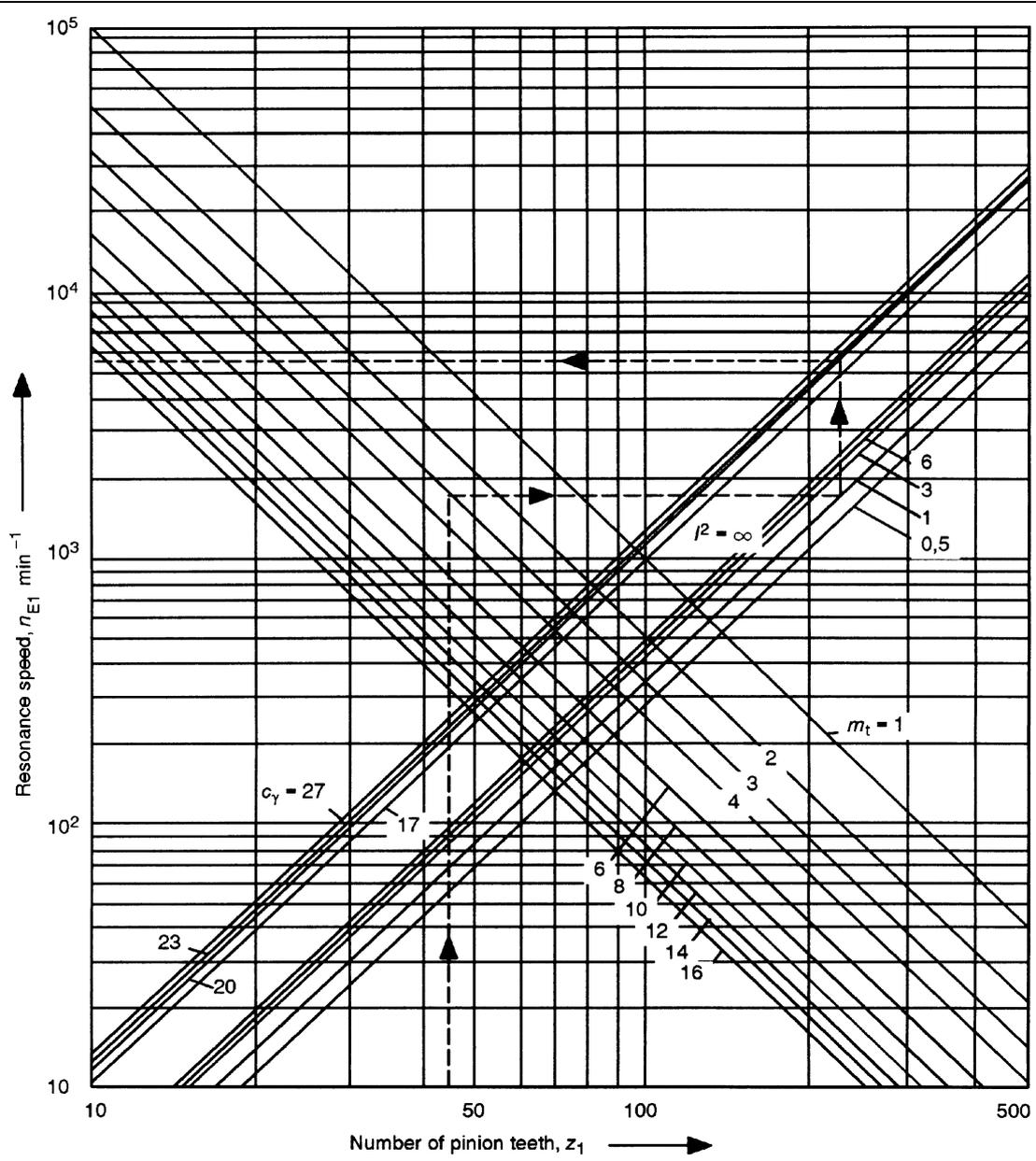
NOTE The pinion being of solid construction with  $q_2$  determined in accordance with equation (28)  $F^2 = (1 - q_2^4) u^2$
