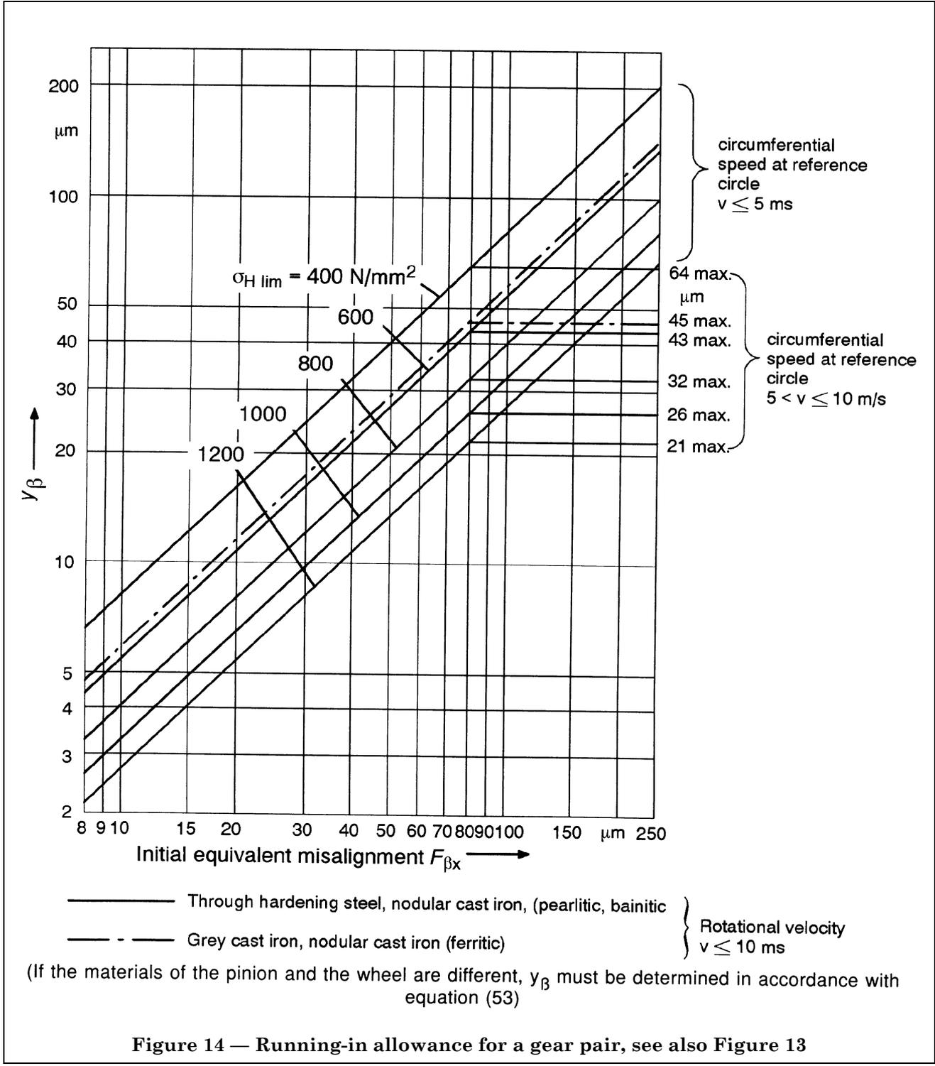
Figure 14 — Running-in allowance for a gear pair, see also Figure 13
