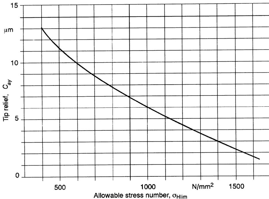
NOTE When the pinion material (1) is different from the wheel (2) then  $C_{ay} = 0.5 (C_{ay1} + C_{ay2})$ .
