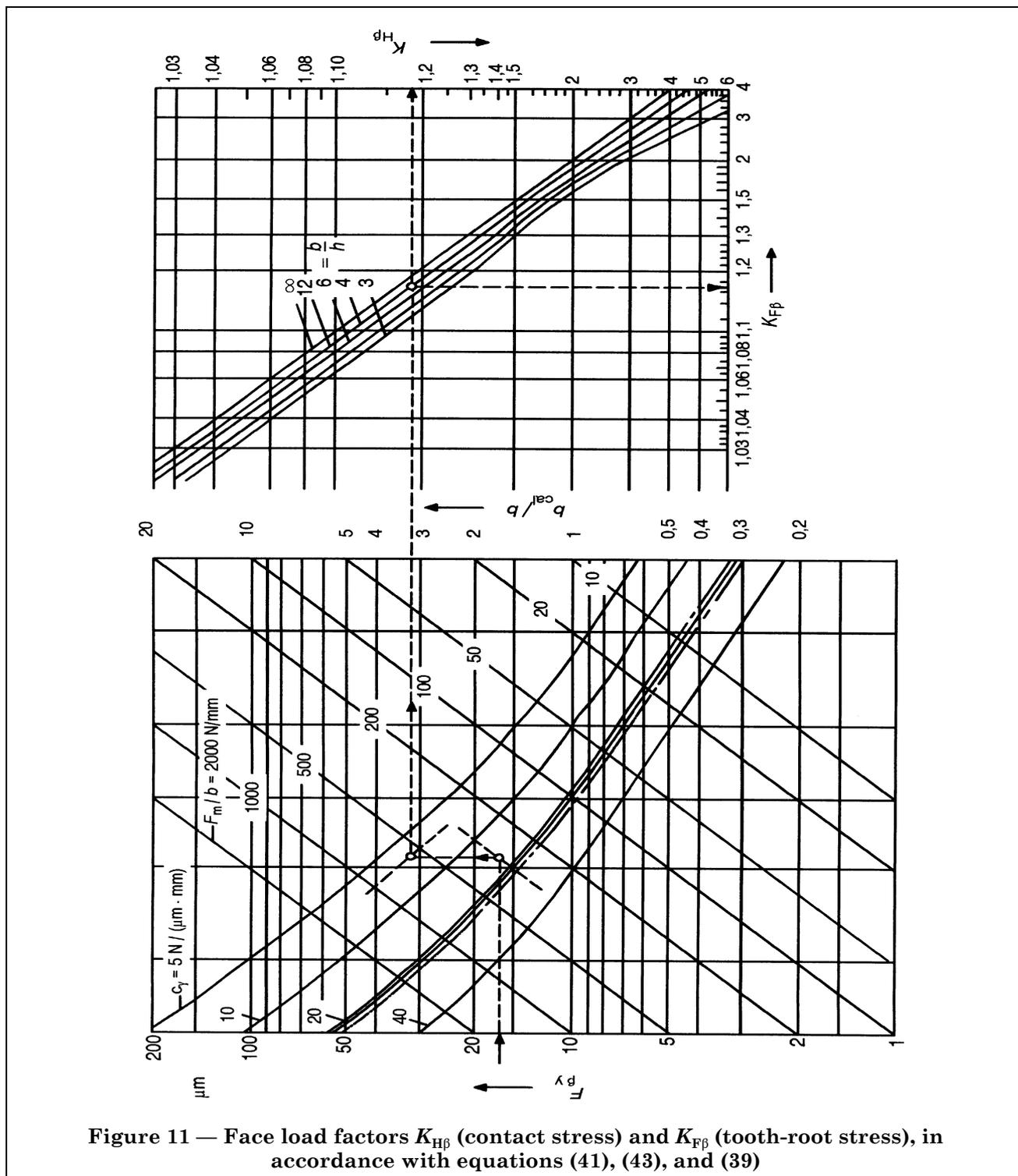
Figure 11 — Face load factors  $K_{H\beta}$  (contact stress) and  $K_{F\beta}$  (tooth-root stress), in accordance with equations (41), (43), and (39)
