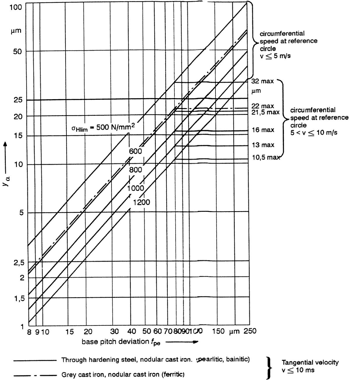
NOTE This graph is derived from Figure 14. If the materials of the pinion and the wheel are different,  $y_\alpha$  shall be determined in accordance with equation (125).
