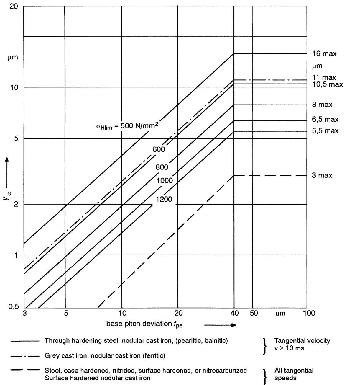
NOTE This graph is derived from Figure 13. If the materials of the pinion and the wheel are different,  $y_{\alpha}$  shall be determined in accordance with equation (125).
