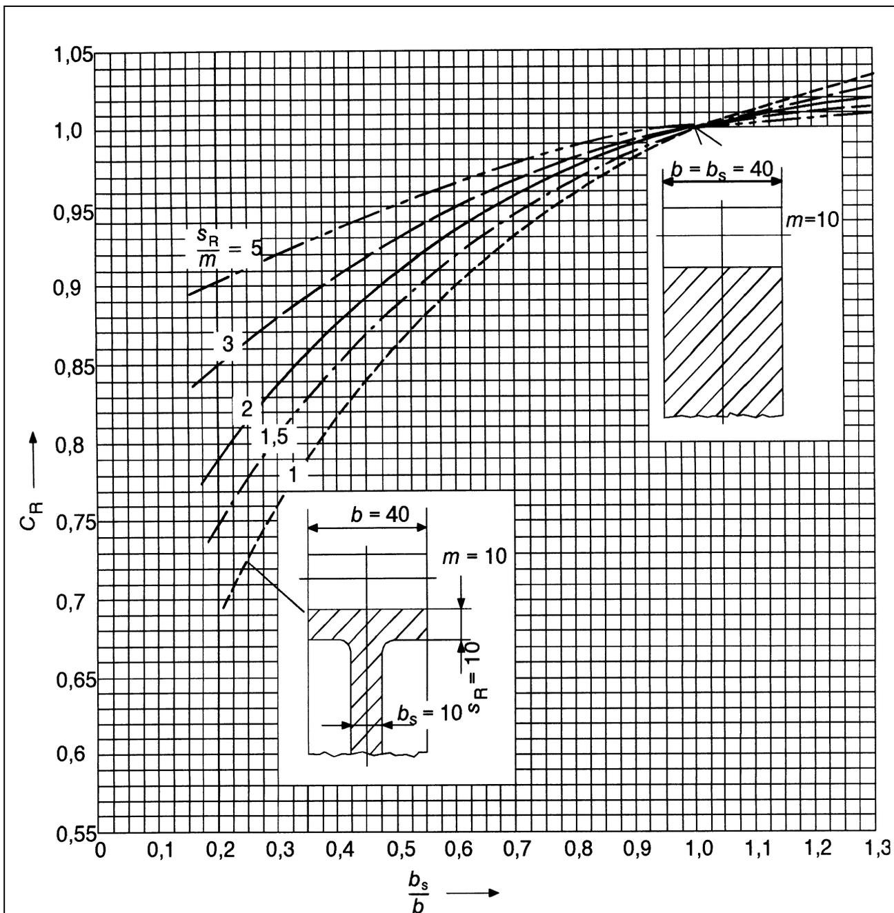
Figure 30 — Wheel blank factor  $C_R$ : mean values for mating gears of similar or stiffer wheel blank design
