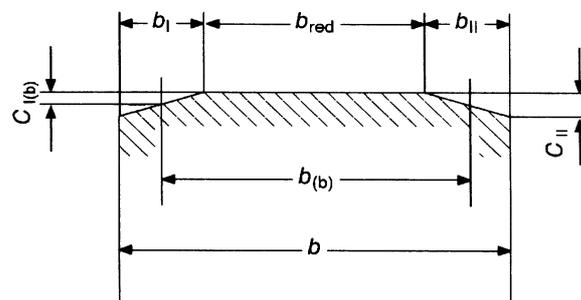
Figure A.2 — Amount  $C_{I(II)(b)}$  and width  $b_{(b)}$  of end relief (see 7.6.2.2)
