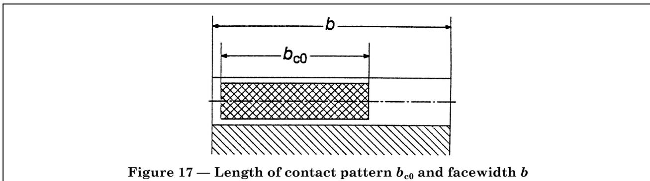
Figure 17 — Length of contact pattern  $b_{c0}$  and facewidth  $b$
