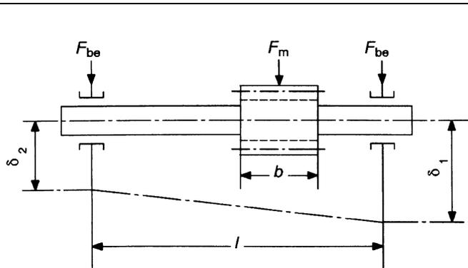
**Figure 18 — Loading and deflections for a gear mounted between the bearings, see equation (100)**
