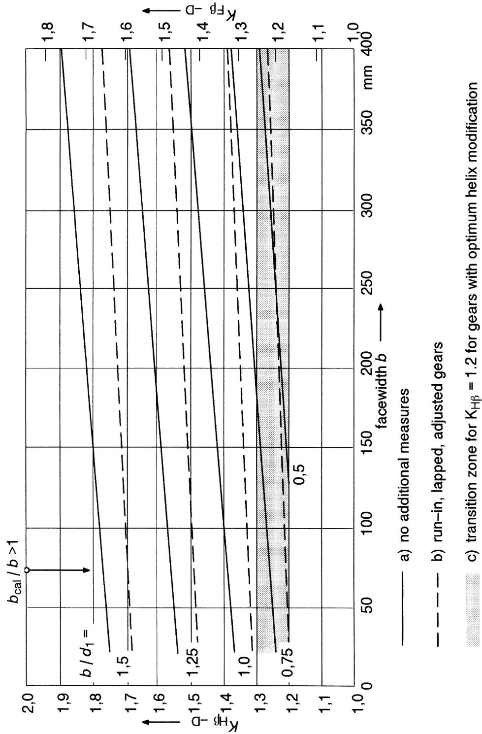
Figure 25 — Curves of face load factors  $K_{H\beta-D}$  and  $K_{F\beta-D}$  for surface hardened cylindrical gears of quality grade 6 according to ISO 1328-1
