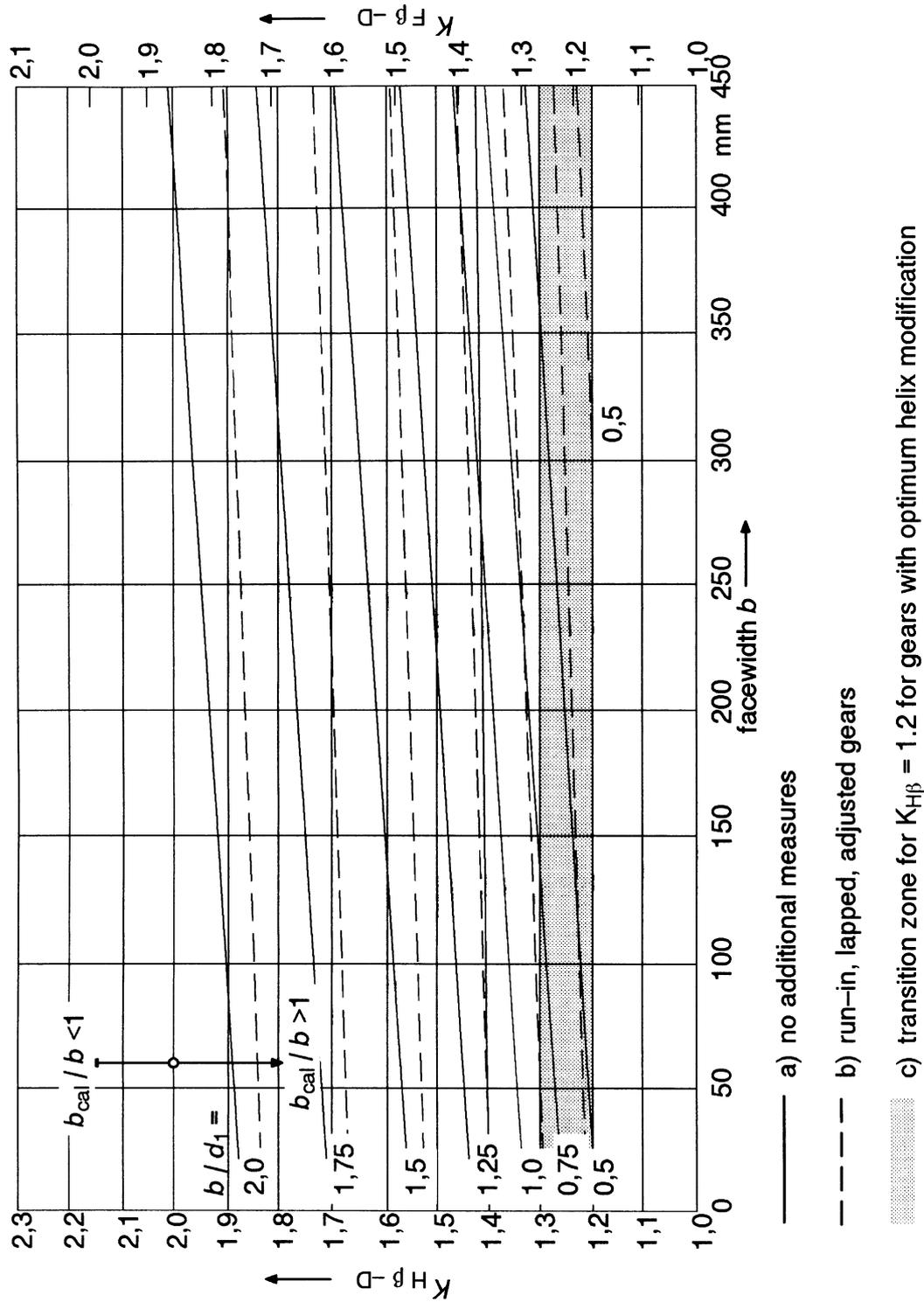
Figure 21 — Curves of face load factors  $K_{H\beta-D}$  and  $K_{F\beta-D}$  for unhardened cylindrical gears of quality grade 6 according to ISO 1328-1
