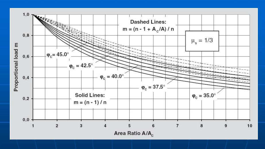
Fig1(d): Proportional Load on Stone Columns for different values of friction angles.
