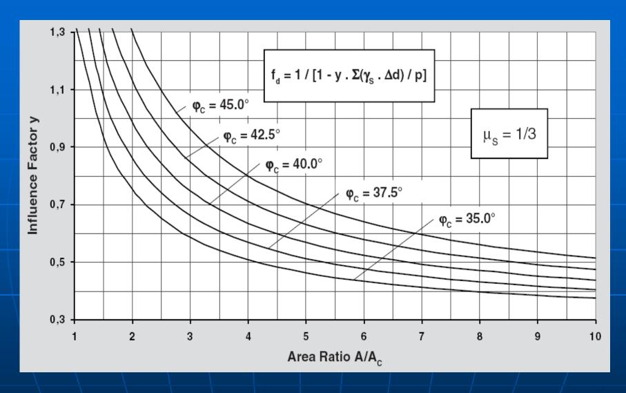
Fig 1(c): Variation of Influence factor, y for different values of friction angles.
