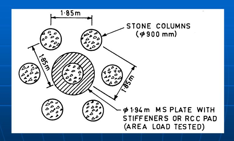
Fig1(d): Load test on single columns.
