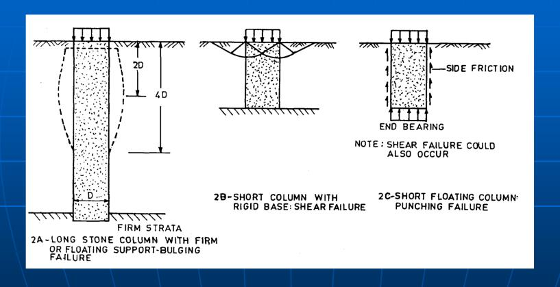
Fig1(a): Failure Mechanism of Single Stone Column in a Homogenous Soft Layer.
