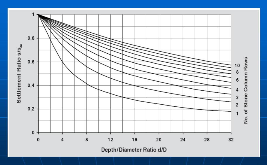
Fig1(f): Variation of settlement ratio with d/D ratio of Strip Footing
