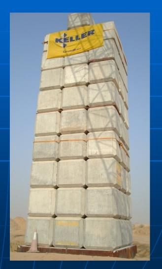
400 Tons load on 4m x 4m ~ 250 kPa
