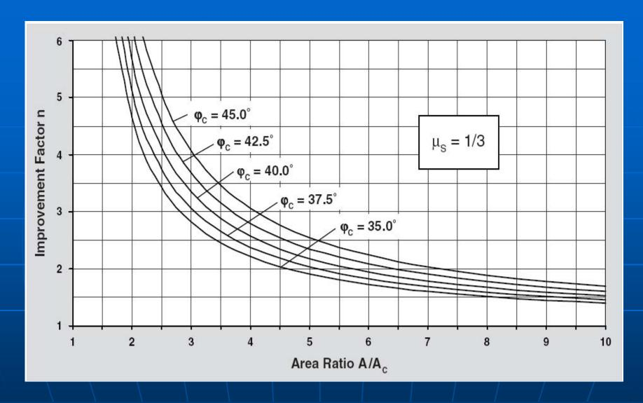
Fig1(a): Relation between the improvement factor  $n_0$ , the reciprocal area ratio A/A<sub>C</sub> and the friction angle of the backfill material,  $\phi_c$ .
