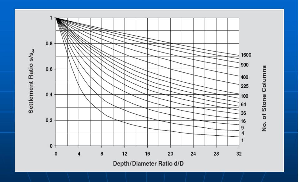
Fig1(e): Variation of settlement ratio with d/D ratio of Single Footing
