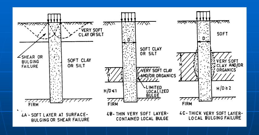
Fig1(b): Failure Mechanism of Single Stone Column in a Non-Homogenous Soft Layer.
