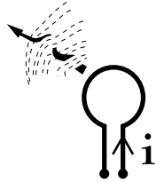
Loop = "transmitting" antenna
