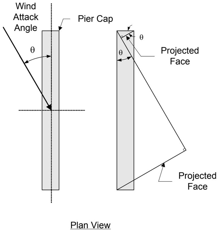
**Figure 8-7 Projected Area for Wind Pressure on Pier**
