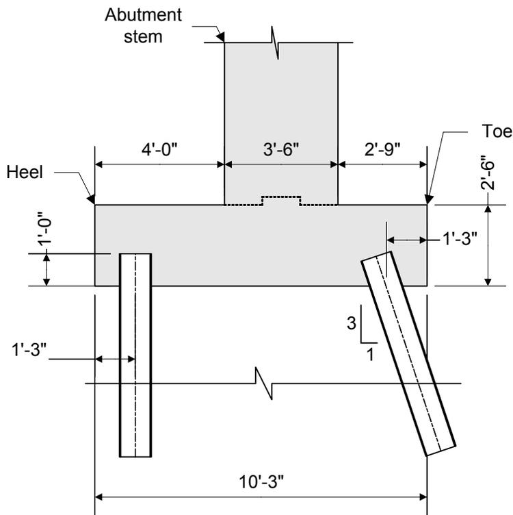
**Figure 7-16 Abutment Footing and Pile Foundation Elevation View**
