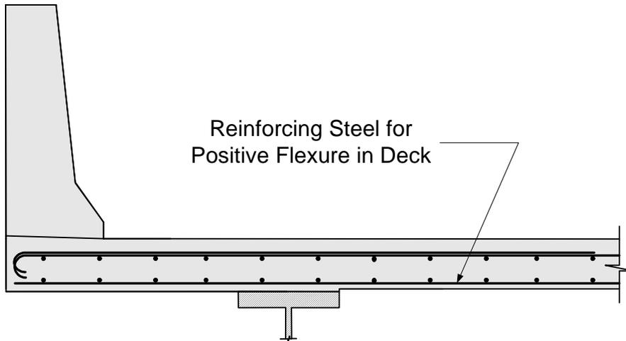
**Figure 2-4 Reinforcing Steel for Positive Flexure in Deck**
