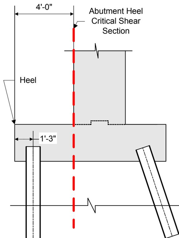
**Figure 7-23 Abutment Heel One-way Action Critical Section**
