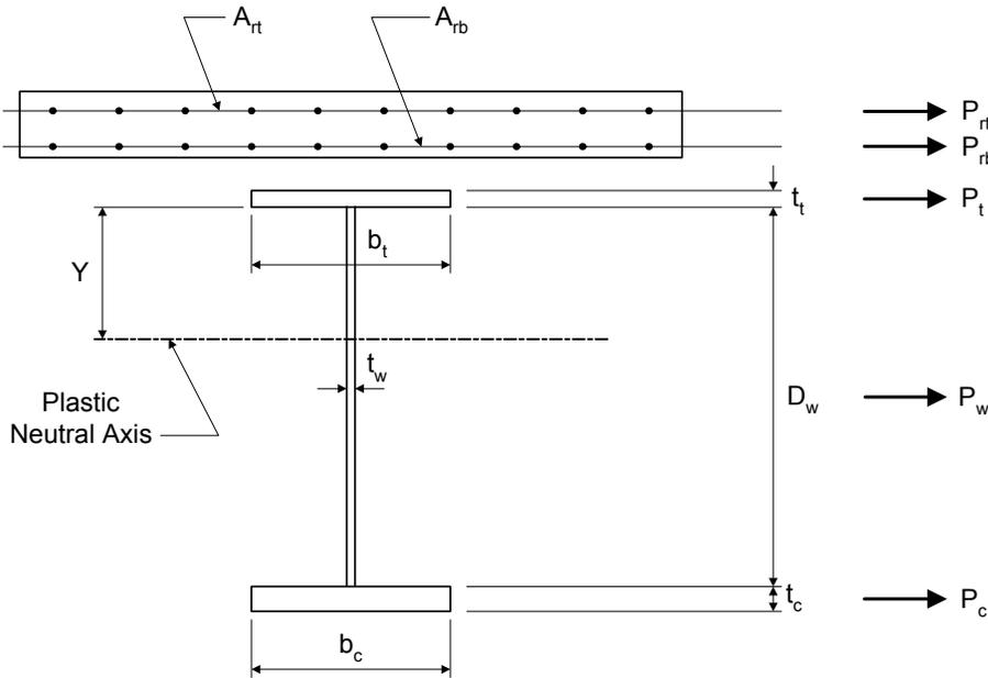
**Figure 3-13 Computation of Plastic Moment Capacity for Negative Bending Sections**
