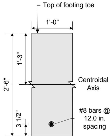
**Figure 7-18 Abutment Footing Toe Cracking Moment Dimensions**
