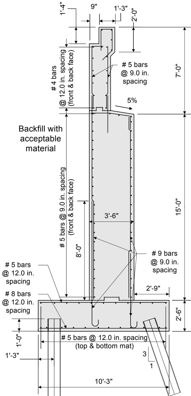
**Figure 7-25 Final Abutment Design**
