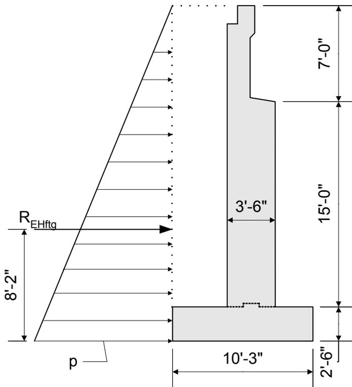
**Figure 7-7 Bottom of Footing Design Earth Load**
