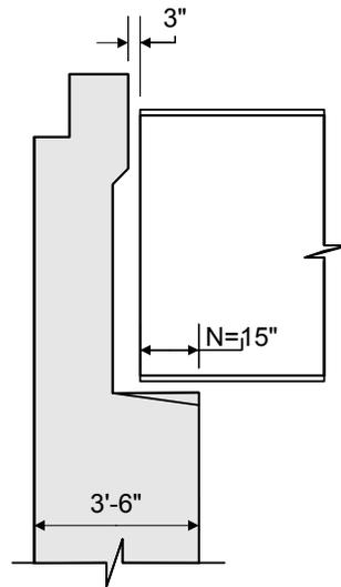
**Figure 7-4 Minimum Support Length Required**
