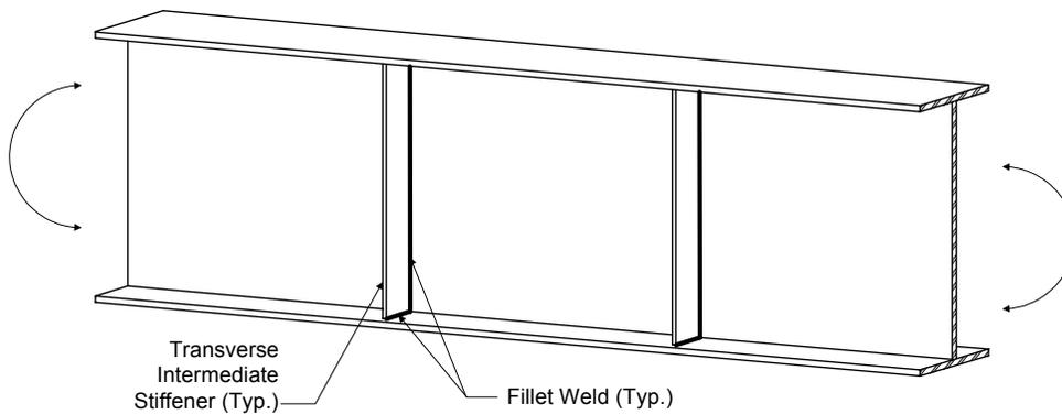
**Figure 3-10 Load-Induced Fatigue Detail**
