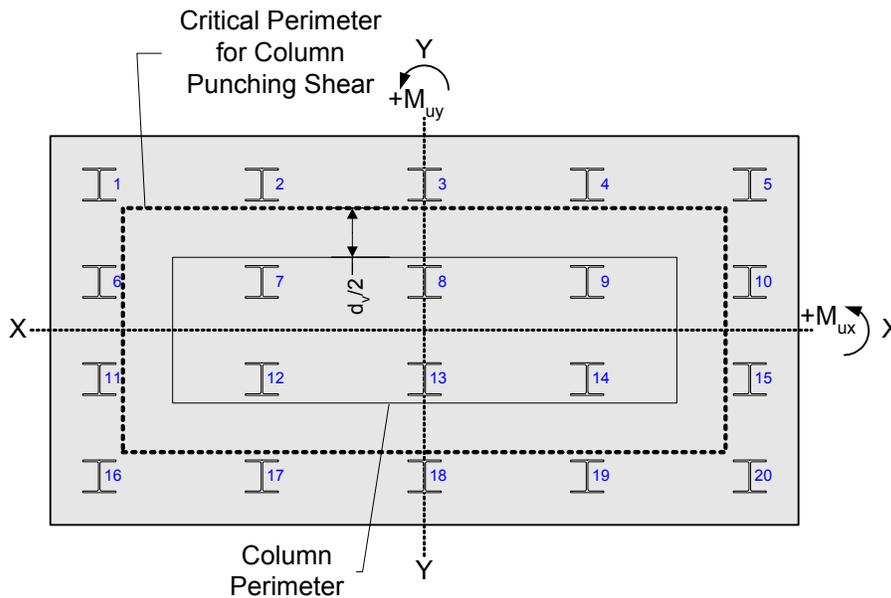
**Figure 8-12 Critical Perimeter for Column Punching Shear**
