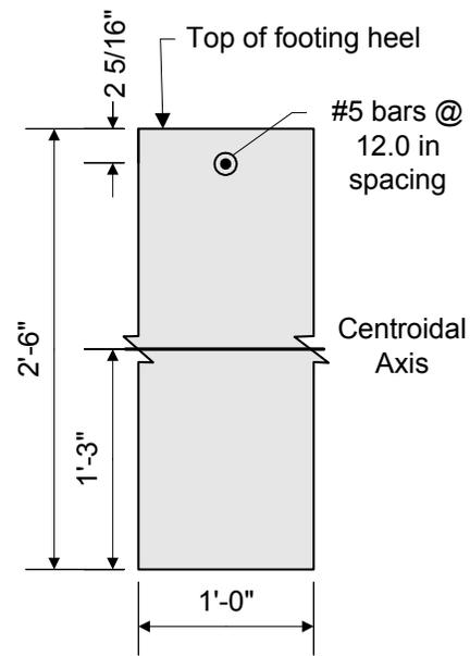
**Figure 7-21 Abutment Footing Heel Cracking Moment Dimensions**
