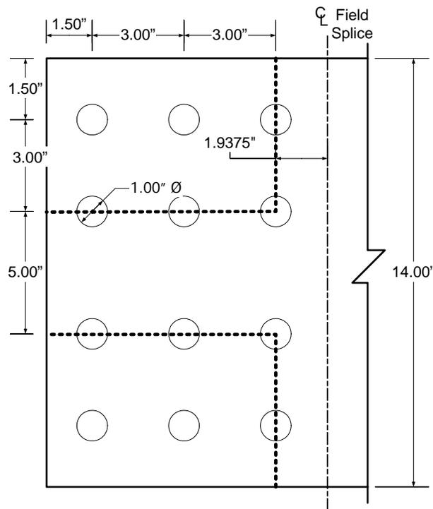
**Figure 4-5 Outside Splice Plate - Failure Mode 2**
