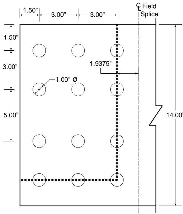
**Figure 4-4 Outside Splice Plate - Failure Mode 1**
