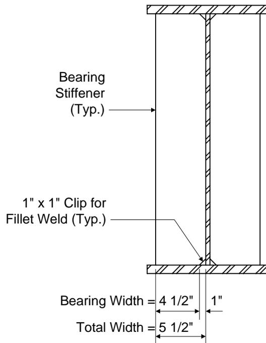
**Figure 5-4 Bearing Width**
