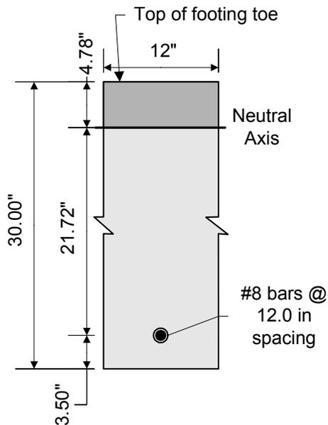
**Figure 7-19 Abutment Footing Toe Crack Control Check**
