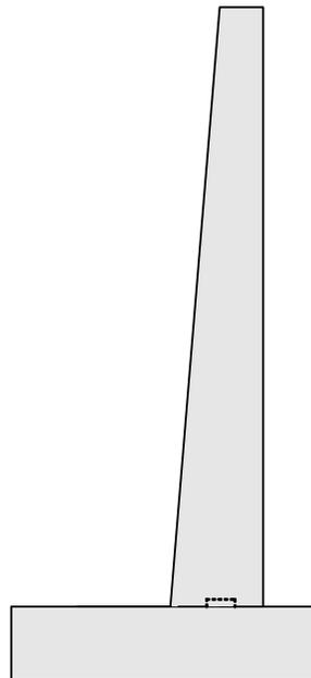
**Figure 7- 26 Reinforced Concrete Cantilever Wingwall**
