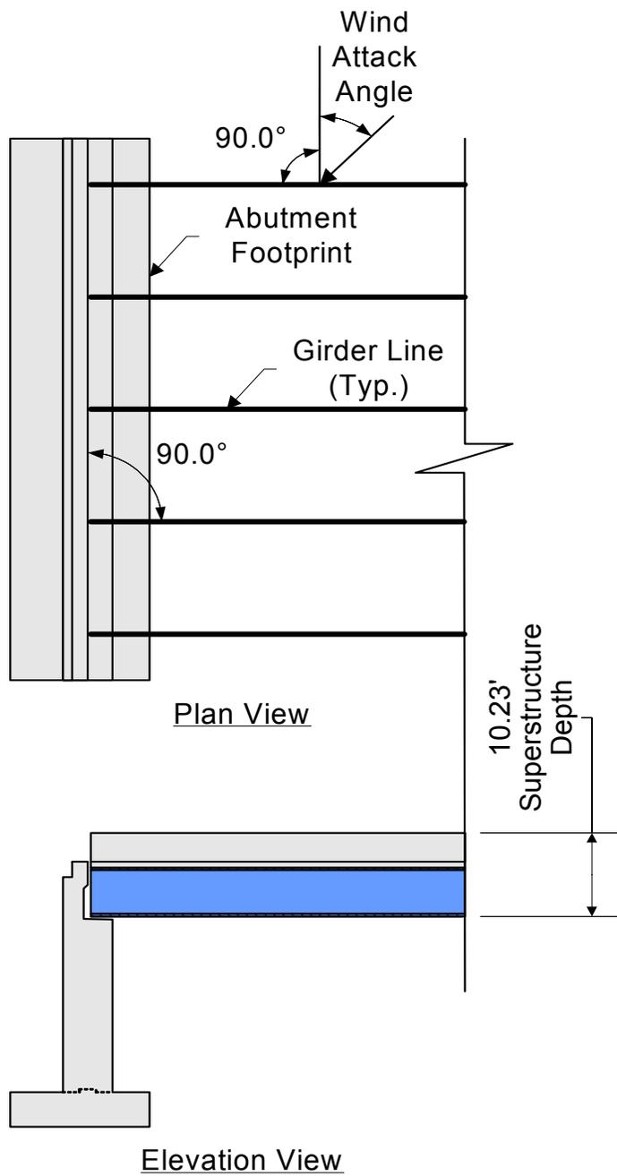
**Figure 7-3 Application of Superstructure Wind Load on Abutment**
