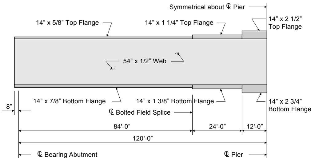
**Figure 3-4 Plate Girder Elevation**
