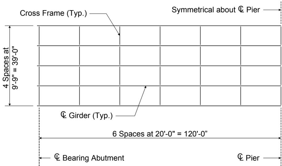
**Figure 3-3 Framing Plan**
