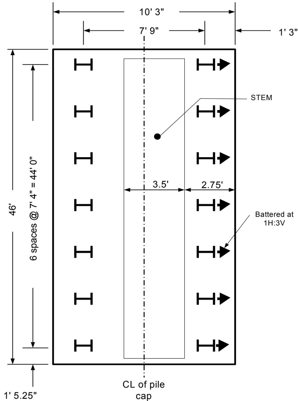
**Figure P-16 Final Pile Cap Layout**
