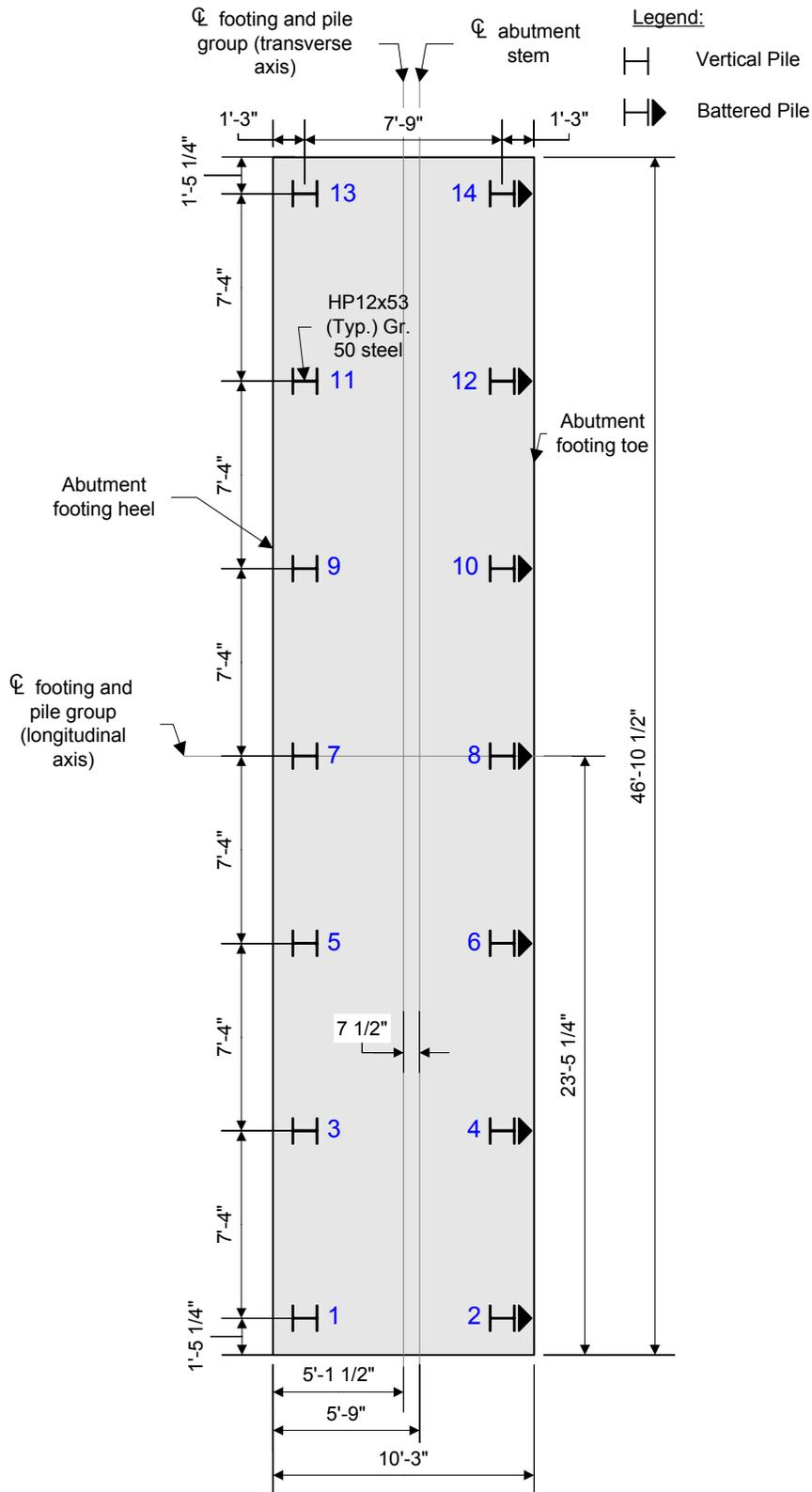
Figure 7-15 Abutment Footing and Pile Foundation Plan View
