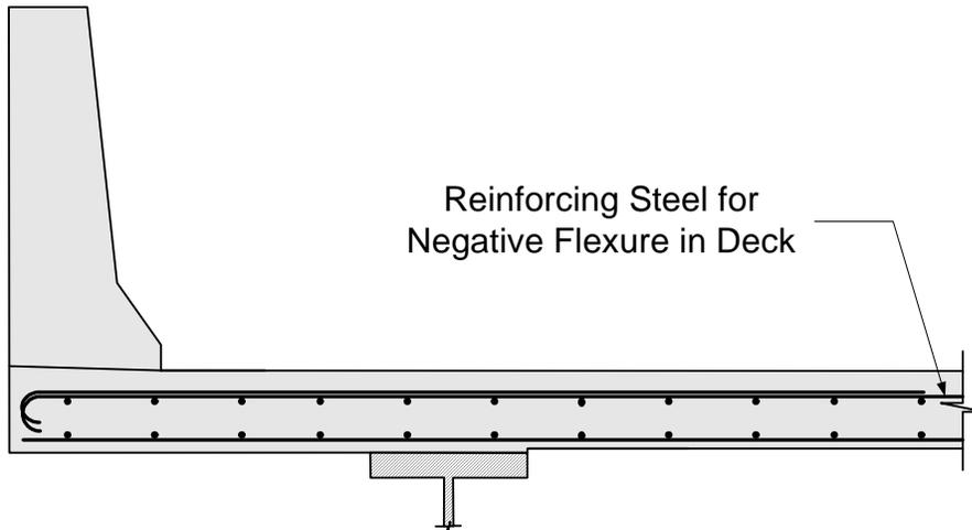
**Figure 2-7 Reinforcing Steel for Negative Flexure in Deck**
