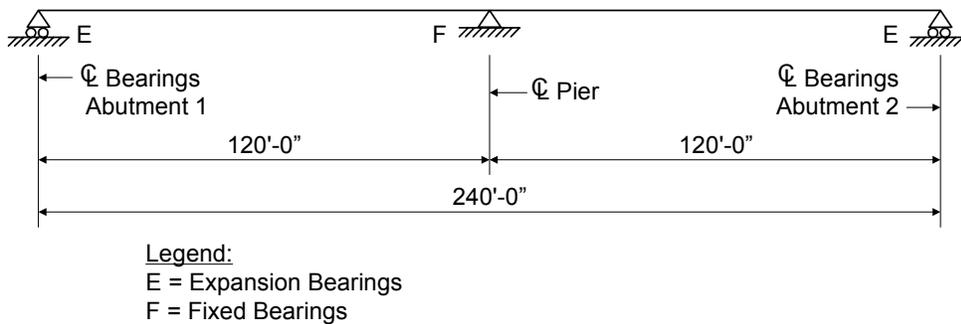
**Figure 1-1 Span Arrangement**
