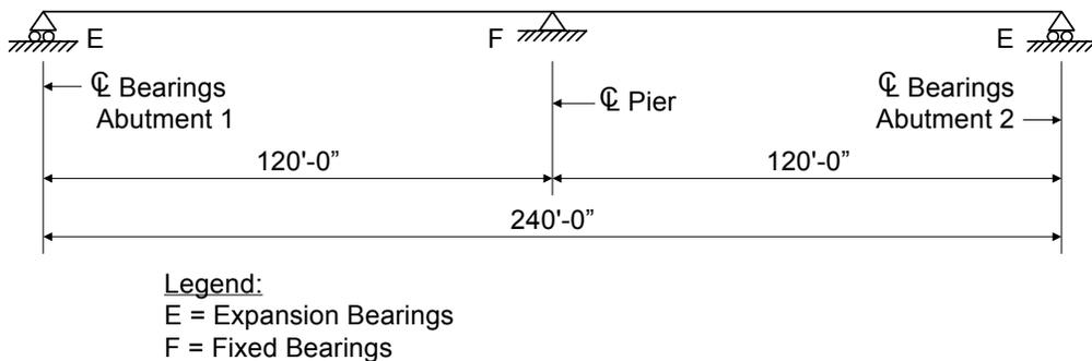
**Figure 3-1 Span Configuration**
