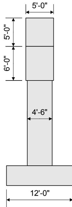
**Figure 8-3 Preliminary Pier Dimensions - End Elevation**
