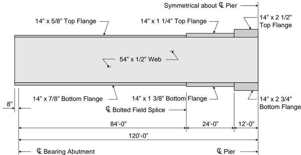
**Figure 4-1 Plate Girder Elevation**
