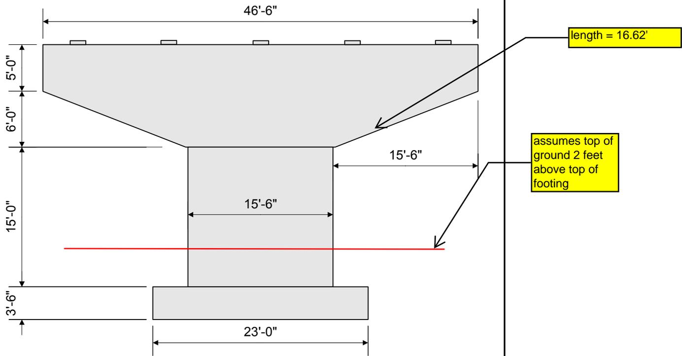
**Figure 8-2 Preliminary Pier Dimensions - Front Elevation**
