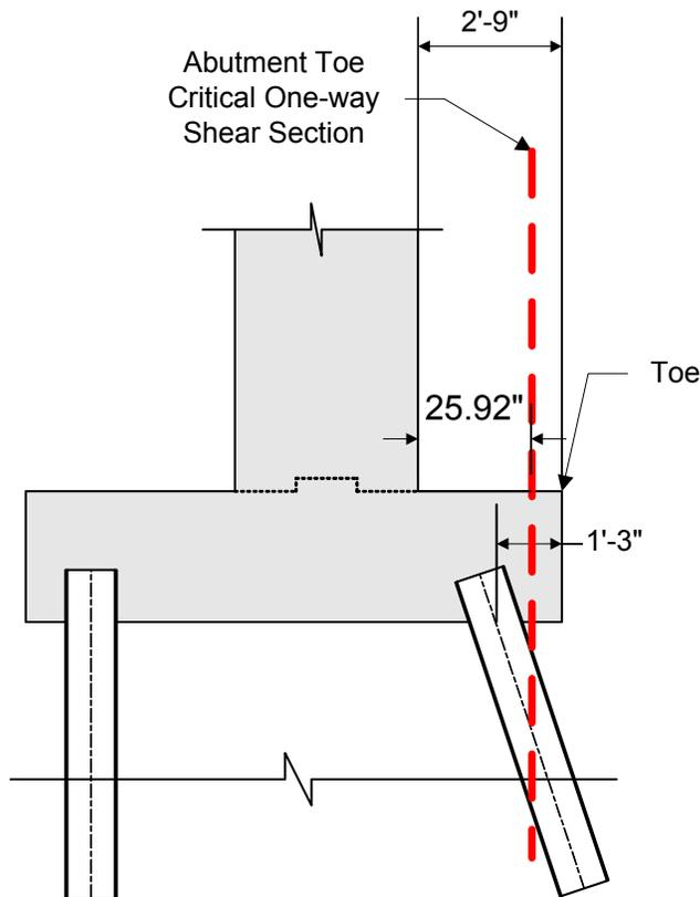
**Figure 7-22 Abutment Toe One-way Action Critical Section**
