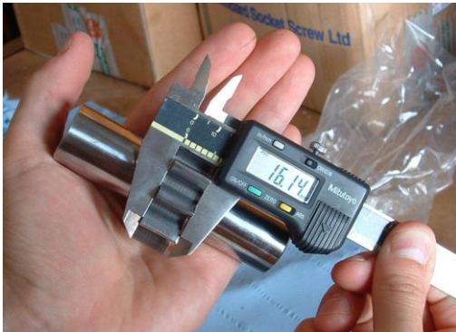
Photo 1 – shows gear width 1.614cm
