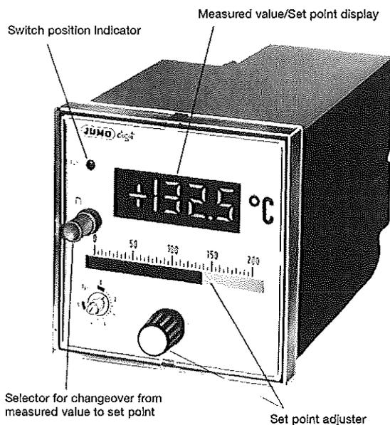
Figure 31 Regulator with digital display
