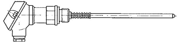
Figure 33 Screw-in type resistance thermometer Pt 100
