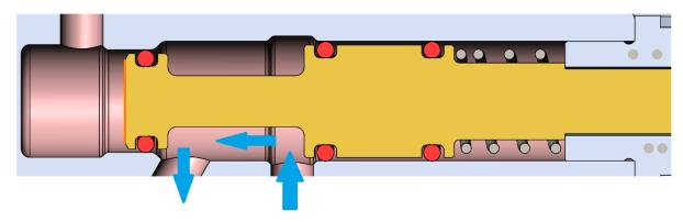
Valve feed closed. 500psi air in small chamber is back purging to atmospheric.
